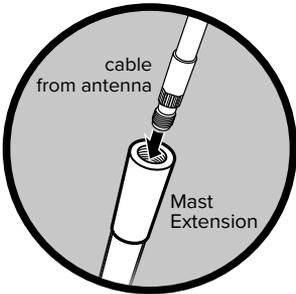
Once you have determined the best location for the antenna and have determined if Mast Extensions are needed, insert cable **through** mast.
