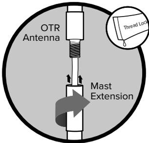
If using Mast Extension(s) add **thread locker** (packets provided) to thread point(s). Screw into place.
