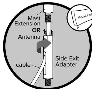
Add thread locker (packets provided) to thread point and screw on the **Side Exit Adapter**.
