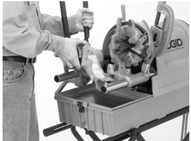
Figure 4 – Mounting on No. 1822-I Threading Machine (Same applies to Models 300 Compact and 535 Threading Machines)
