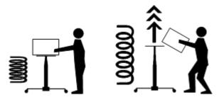
Do not unplug the hose and hand control with a load on the platform. Be aware of the position of the hose and hand control and protect it from puncture, crushing and severing.
