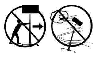
Do not operate the machine in strong or gusty winds. Increasing the load surface area will decrease machine stability in windy conditions.
