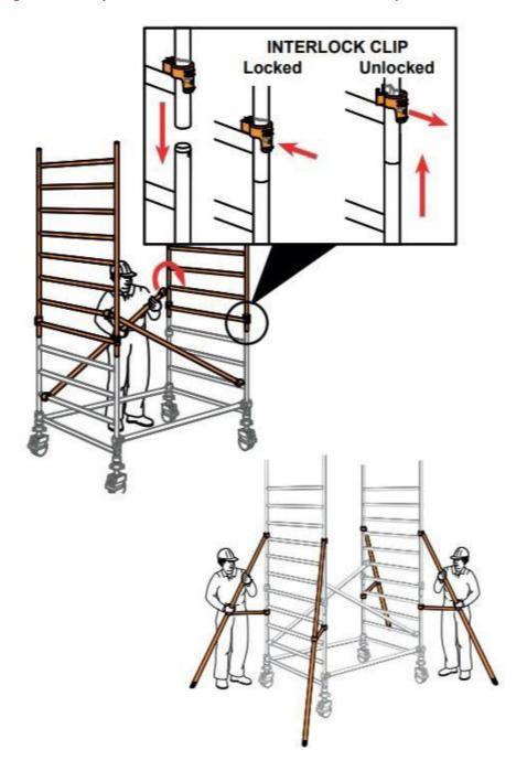
5. Fit a temporary deck on the lowest rungs. Fit a trapdoor deck on the 8th rung (2.0m) on one side of the tower. Ensure that the trapdoor is positioned with the hinges towards the outside of the tower as shown. Climb the end frame below the trapdoor on the inside of the tower, and from within the protected trapdoor position, fit horizontal braces on the 10th and 12th rungs (in that order) on both sides of the deck. Do not climb onto the deck until all guardrails are in place.
