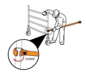
2. Position the second end frame as shown and fit the other end of the horizontal brace on to the vertical, just above the bottom rung. Fit a second horizontal brace on the bottom rungs on the other side of the frames to square the tower.
