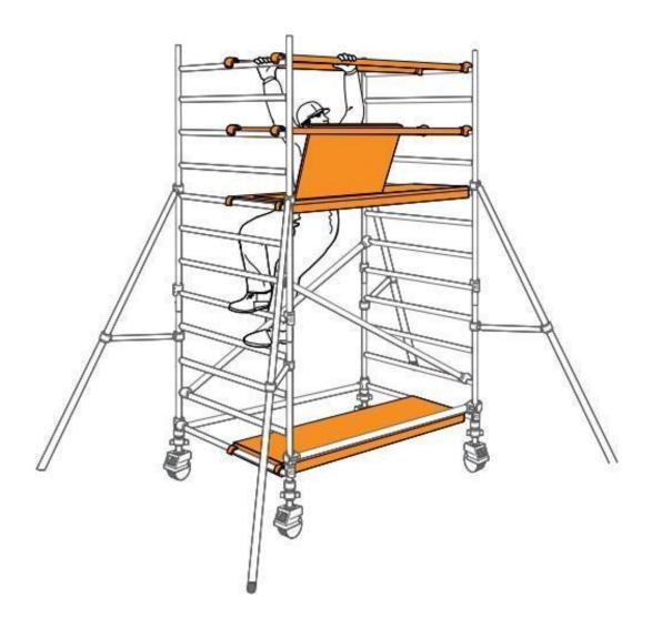
6. Fit the next pair of diagonal braces in opposing directions between the 6th and 10th rungs add two additional end frames.
