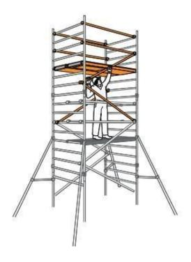
8. Continue to add pairs of end frames, diagonal braces and fit trapdoor decks as shown in the previous steps. At every platform level, add horizontal braces as guardrails at 2 and 4 rungs above the platform. Fit these guardrail braces from the protected trapdoor position. Do not climb onto the platform until all guardrails are in place.
