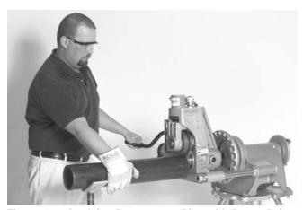
Figure 16 – Applying Pressure on Pipe with Power Drive in REV Mode.
