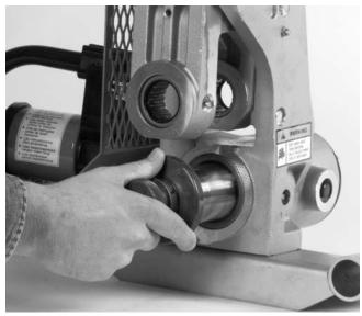
Figure 20 - Removing Drive Shaft
