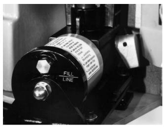
Figure 24 - Reservoir Filler Cap
