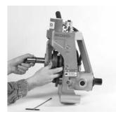
Figure 18 – Removing Retaining Shaft and Groove Roll
