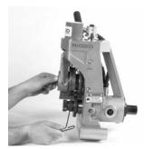
Figure 17 – Loosening Grooving Roll Set Screw
