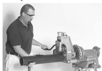
Figure 15 – Applying Pressure on Pipe with Power Drive in FORWARD Mode
