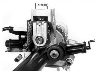
Figure 23 - Stabilizer Positioning
