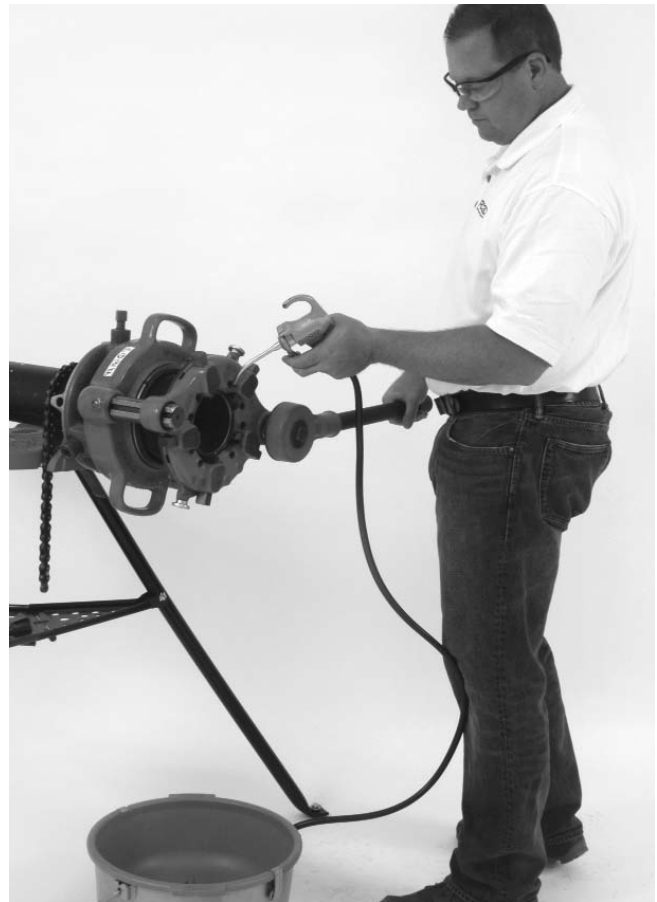
Figure 7 – D-1440 Ratchet Operation
