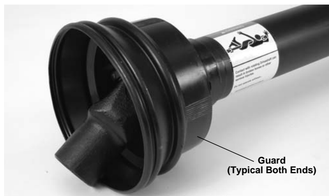
Figure 9 – 840A Driveshaft Guard and Warning
