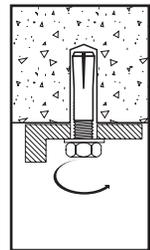
If using a fixture, position it, insert bolt and tighten. Most overhead applications typically utilize threaded rod. Minimum thread engagement should be at least one anchor diameter.
