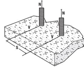
**Edge Distance, Tension ( $F_{NC}$ ) (Normal-Weight concrete only)**
