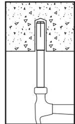
Using a DEWALT setting tool specifically, set the anchor by driving the tool with a sufficient number of hammer blows until the shoulder of the tool is seated against the anchor. Note: anchor will not hold published load if shoulder of DEWALT setting tool does not seat against anchor.
