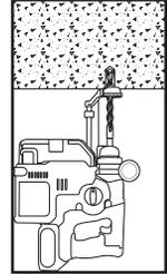
Remove dust and debris from the hole during drilling (e.g. dust extractor, hollow bit) or following drilling (e.g. suction, forced air) to extract loose particles created by drilling. Insert the anchor into the hole and tap flush with surface.
