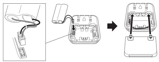
• The battery harness plug has a large notch on it that faces to the left away from the Gas Alarm when installed correctly. There is only one way in which the plug can be installed. A small portion of the plug will be exposed when connected properly.
