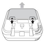
• Connect the batteries by inserting the battery harness plug into the Gas Alarm receptacle as shown in the diagram below. **Do NOT remove the plastic wrap** surrounding the batteries.
