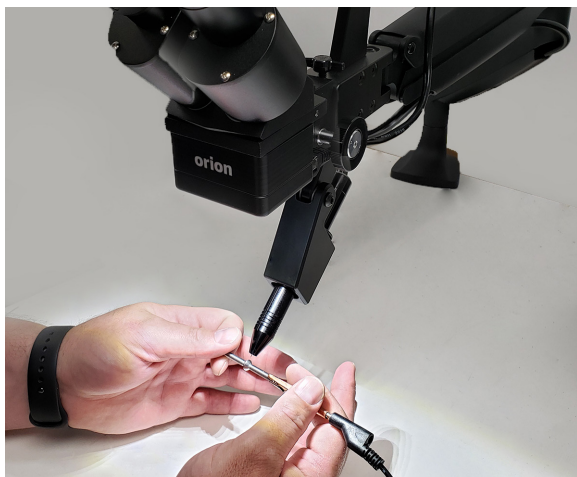
Figure 10.1. Rest your hands on the table and position the workpiece close to, but not touching the electrode. Then look through the microscope.
