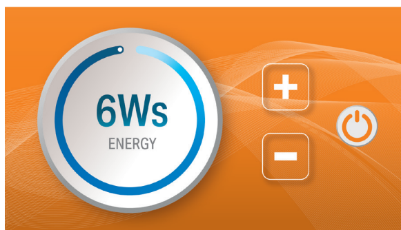
Figure 14.1 Set the Weld Energy Level to 7 ws and then tap the Weld On/Off button so the power icon changes color from gray to orange.
