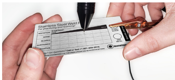
Figure 14.2 Attach the alligator clip to the welding plate. With proper eye protection, hold the welding plate with both hands and lightly touch the electrode to the welding plate. When the electrode contacts the welding plate, the welder will release energy and create a weld.
