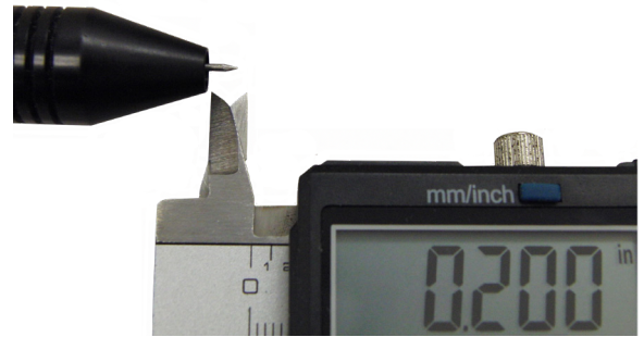
Figure 7.1. Electrodes should protrude past the stylus hull 1/8 to 1/4 inch (3.175 to 6.35mm).
