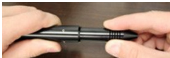
Figure 6.2. To install the electrode, first remove the Stylus Shaft (A) from the Stylus Hull (E) by pulling them apart.
