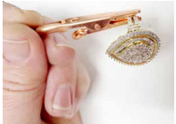
Figure 19.2. Attach the alligator clip ground to the workpiece at a spot that ensure the best contact between ground and workpiece.
