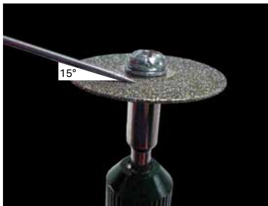
Figure 8.2. Use a rotary tool to sharpen the electrode.
