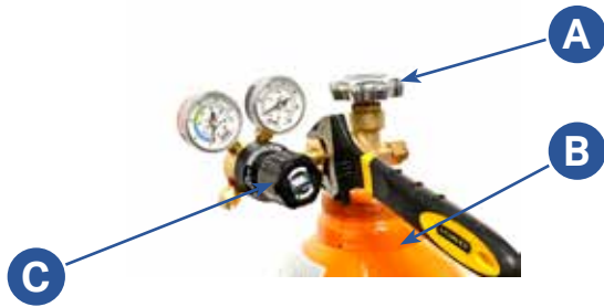
Figure 10.1. First, turn the regulator dial (C) counterclockwise to close the regulator valve. Screw the gas regulator (A) to the top of the shielding gas tank (B).
