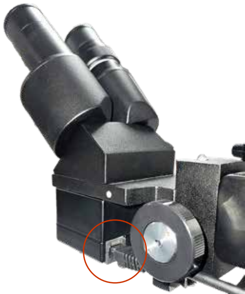
Figure 4.3 After installing the rubber eyepiece covers, use the Shutter Cable to connect the power supply to the bottom of the microscope head.
