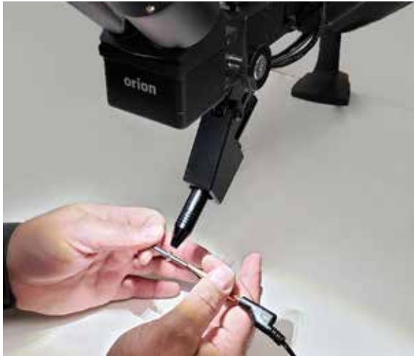
Figure 12.1. Rest your hands on the table and position the workpiece close to, but not touching the electrode., Then look through the microscope.
