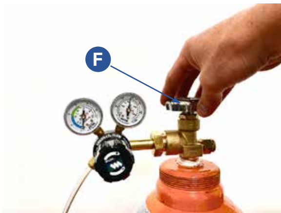
Figure 10.3. Open the shielding gas tank main valve (F) slowly clockwise until the left dial on the regulator port indicates gas pressure of 7-10 liters per minute.
