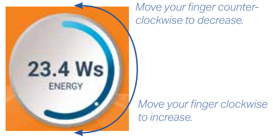
Figure 19.1. The white wheel is used for adjusting energy, length, and rate of fire.
