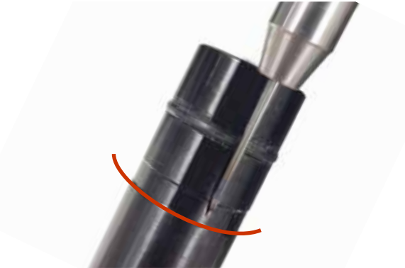
Figure 6.2. Use the guide engraved on the side of the stylus hull (E) for proper electrode (D) positioning.
