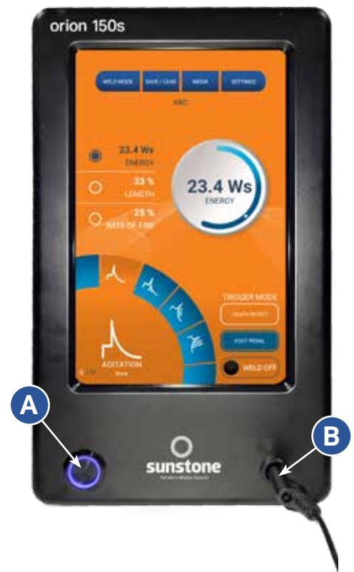
Figure 13.1. To get started, press the Power Button (A); wait for the software to load; insert the alligator clip ground (B).
