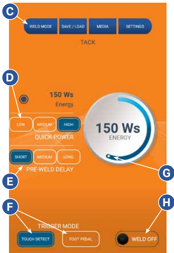
Figure 20.1. To weld in Tack Mode, first attach grounds to the back panel as shown in Figure 20.2; select the desired Quick Power (D); select the desired Pre-Weld Delay (E); select the desired Trigger Mode (F); press the Weld Off Button (H) to toggle to Weld On Mode.
