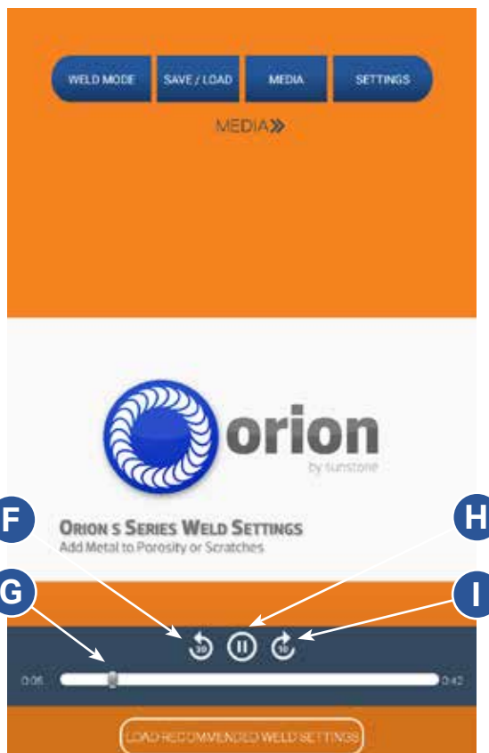
Figure 36.2. To play a video, press the Play Button (H). To rewind by 30 seconds, press the Rewind 30 Button (F). To fast forward by 10 seconds, press the Forward 10 Button (I). Use the slider bar (G) to find any point in the video.
