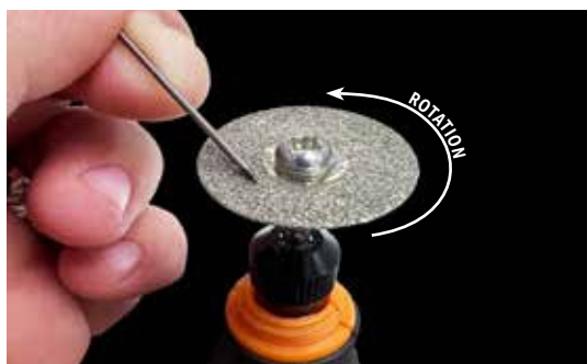
Figure 8.1. A sharp electrode tip improves arc initiation and results in a better overall weld.
