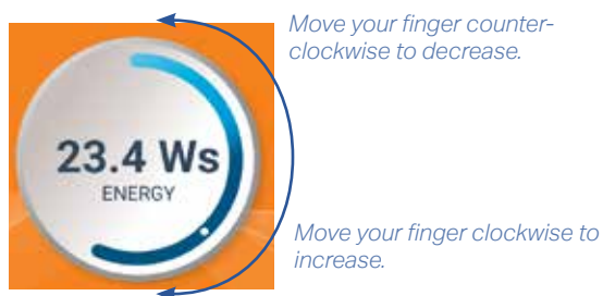
Figure 14.2. The white wheel is used for adjusting energy, length, and rate of fire.
