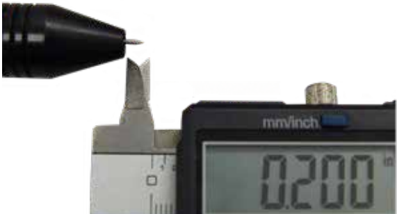
Figure 6.3. The electrode should protrude past the stylus hull (E) 1/8 to 1/4 inch (3.175 to 6.35mm).
