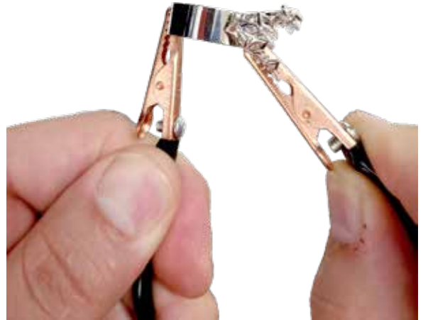
Figure 21.2. To weld in Tack Mode, grounds are attached to two different workpieces. Position the workpieces as desired and then initiate a weld by touch or foot pedal.
