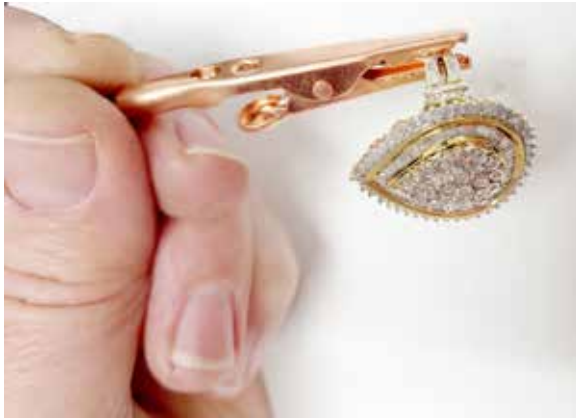
Figure 16.1. Attach the alligator clip ground to the workpiece at a spot that ensures the best contact between ground and workpiece.
