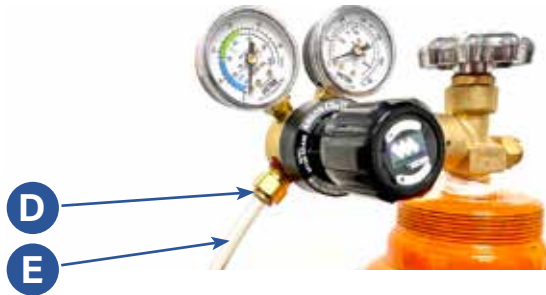
Figure 10.2. Connect the OD gas tube (E) from the power supply to the gas regulator port (D).
