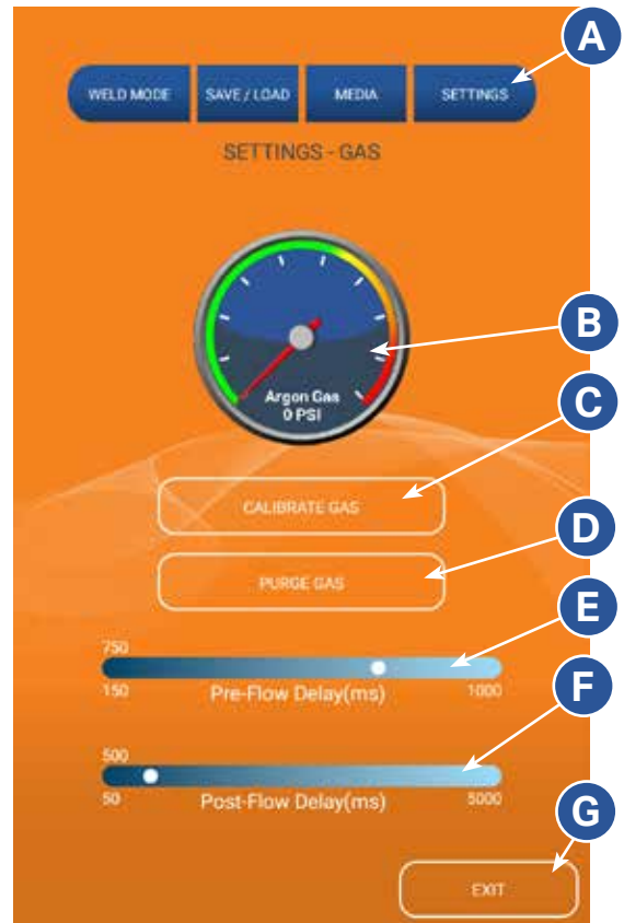
Figure 25.1. Press the Settings Button in the top row blue menu buttons and choose the Gas Screen option to view the current gas pressure (B); to calibrate the gas pressure (C); to purge the gas line (D); to make changes to the pre-flow delay (E); or to make changes to the post-flow delay (F).
