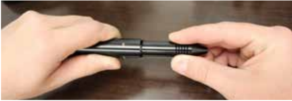
Figure 6.1. To install the electrode, first remove the stylus shaft (A) from the stylus hull (E) by pulling them apart.
