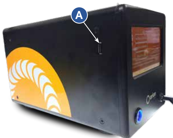
Figure 26.1. To begin to update the welder's software, insert a USB thumb drive containing the software update file in the USB port (A) found on the left side of the welder. Then press the Update Welder Button and follow the on-screen instructions.
