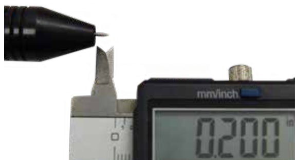
Figure 6.3. The electrode should protrude past the stylus hull (E) 1/8 to 1/4 inch (3.175 to 6.35mm).
