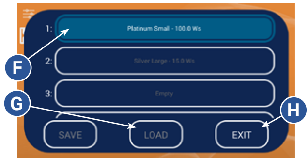
Figure 29.2. To load a weld schedule, find and press the weld schedule you wish to load (for example, F) and then press the Load Button (G). Press the Exit Button (H) to return to the previous screen.
