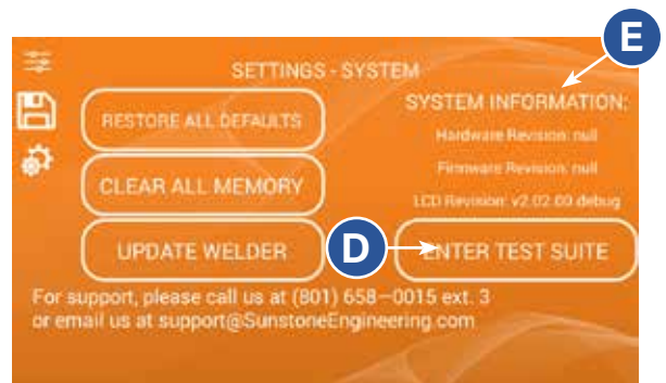
Figure 27.2. In the Settings-System Screen, press the Enter Test Suite Button (D) to enter the test suite for diagnostic purposes.
