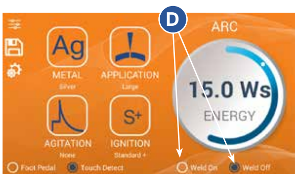
Figure 16.3. Touch the Weld On radio button to begin welding. Touch the Weld Off radio button to avoid an unintentional discharge of energy.
