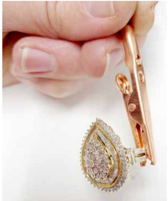
Figure 17.1. Attach the alligator clip ground to the workpiece at a spot that ensure the best contact between ground and workpiece.
