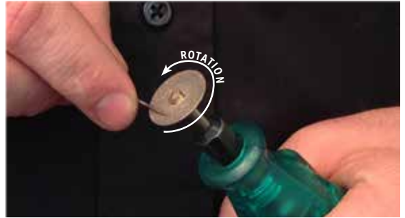
Figure 7.1. A sharp electrode tip improves arc initiation and results in a better overall weld.
