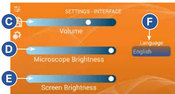
Figure 20.2. Access the Settings-Interface Screen to adjust volume (C), microscope brightness (D), screen brightness (E), and language preferences (F).
