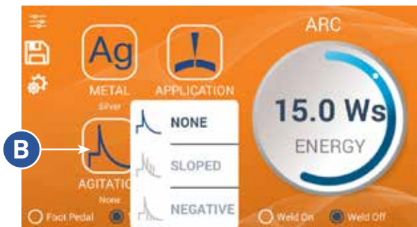
Figure 14.2. To adjust the agitation, press the Agitation Button (B) and choose the desired agitation type.
