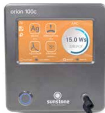
Figure 12.3. Insert the alligator clip to the front of the welder, as shown here.
