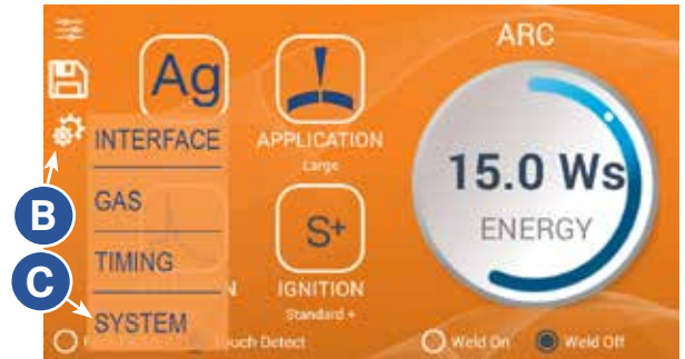
Figure 27.1. To make system-wide changes, press the System Settings icon (B) and then choose System (C) from the sub-menu.
