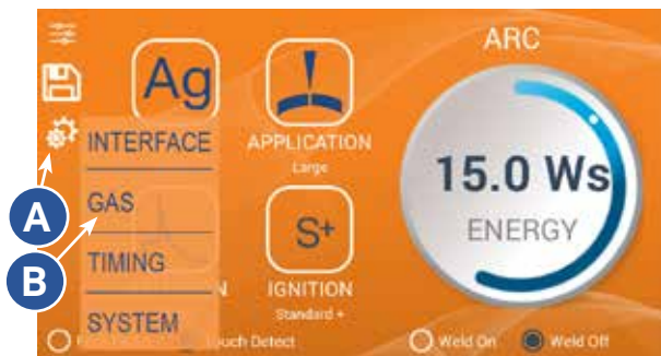
Figure 22.1. To make adjustments to the welder's systems, press the System Settings icon (A) and then choose an option from the sub-menu.
