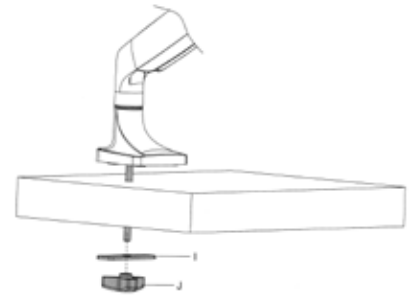
Figure 3.2. Lower the arm so the bolt goes through the hole in the table. Turn the twist knob clockwise to tighten the plate to the table.
