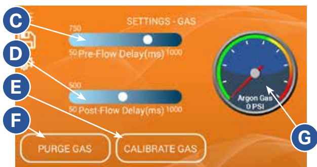
Figure 22.2. Access the Settings-Gas Screen to make adjustments to Pre- and Post-Flow Delays (C and D), to purge gas from the system (F), to calibrate the gas system (E), or to monitor gas pressure (G).
