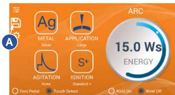
Figure 28.1. To save or load a weld schedule, press the Save/Load icon (A).
