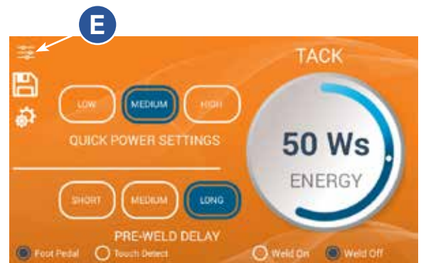
Figure 17.2. Press the Weld Mode icon (E) and choose Tack from the drop down menu.
