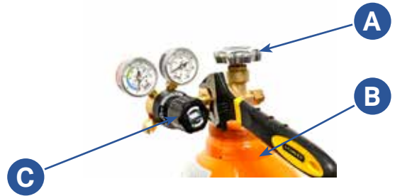
Figure 9.1. First, turn the regulator dial (C) counterclockwise to close the regulator valve. Screw the gas regulator (A) to the top of the shielding gas tank (B).
