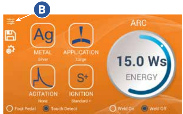
Figure 13.1. To get started, choose the Weld Mode icon (A) and choose Arc or Tack from the drop down menu. The selected weld mode is displayed above the white power selection wheel.
