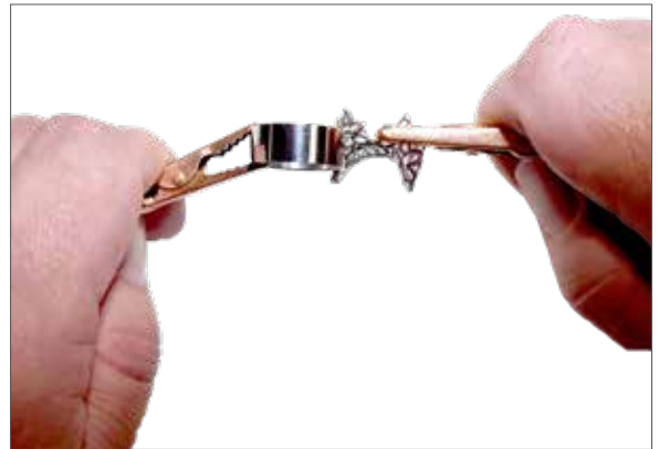
Figure 19.1. To connect the two pieces in Tack Mode, slowly bring the two pieces together. If using a foot pedal, when the two pieces connect, depress the foot pedal and release. If using the Touch Detect Mode, when the two pieces connect a weld will be initiated.
