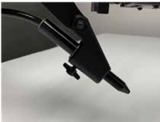
Figure 4.3. Mount the Welding Stylus to the holder below the microscope.
