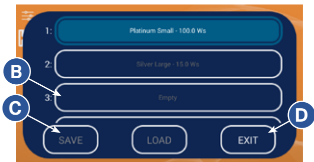
Figure 28.2. To save a weld schedule, press any weld schedule box labeled "Empty" (B) and then press the Save Button (C). Press the Exit Button (D) to return to the previous screen.
