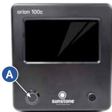
Figure 12.1. Turn the power on by pressing the Power Button (A).
