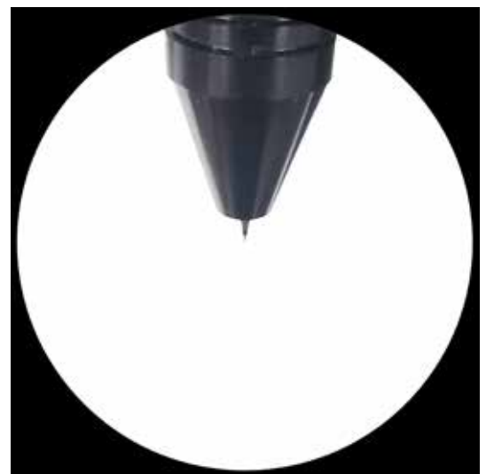
Figure 5.2. Only a small portion of the electrode should extrude from the holder.
