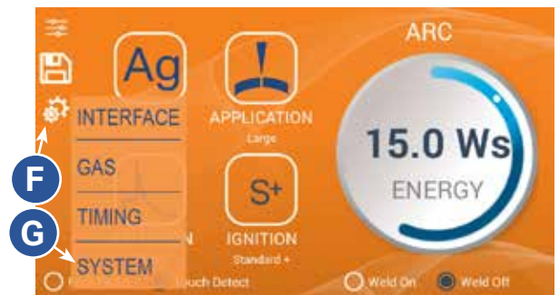
Figure 25.1. To make system-wide changes, press the System Settings icon (F) and then choose System (G) from the sub-menu.
