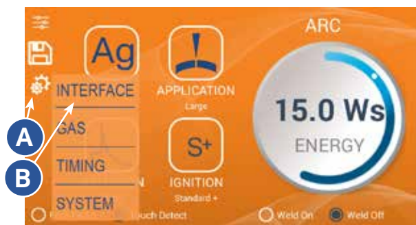
Figure 20.1. To make adjustments to the welder's systems, press the System Settings icon (A) and then choose an option from the sub-menu.
