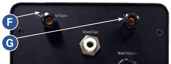
Figure 17.3. Tack Mode requires two grounds attached to the back of the welder, one attached to the Pulse Arc Tack + terminal (F) and the other attached to the Tack - terminal (G).
