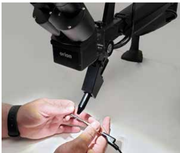
Figure 10.1. Rest your hands on the table and position the workpiece close to, but not touching the electrode., then look through the microscope.
