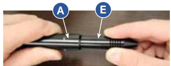
Figure 5.3. To install the electrode, first remove the stylus shaft (A) from the stylus hull (E) by pulling them apart.
