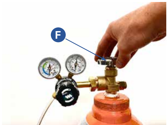
Figure 9.3. Open the shielding gas tank main valve (F) slowly clockwise until the left dial on the regulator port indicates gas pressure of 7-10 liters per second.
