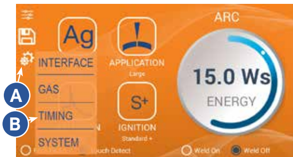
Figure 24.1. To make adjustments to the specific timings, press the System Settings icon (A) and then choose Timing (B) from the sub-menu.
