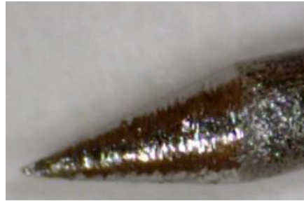
Figure 17.2. Grinding the electrode such that circular rings or marks show up will lead to poor weld quality.
