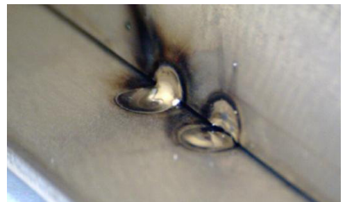
Figure 19.2. A sharp electrode will help place the weld into tight geometries, a blunt electrode can spread the energy and prevent weld formation.
