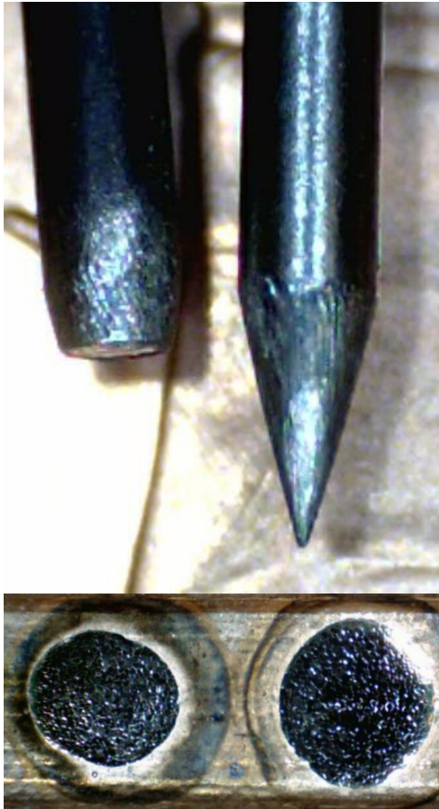
Figure 18.1. The tip shape changes the energy focus and weld penetration, as shown above.
