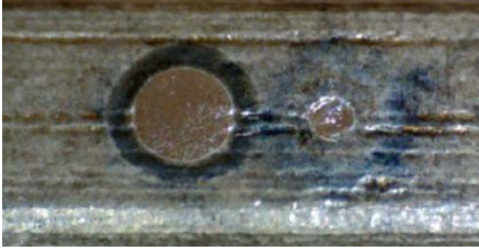
Figure 10.2. The impact of weld length can be seen here. Both welds used the same amount of energy but for different durations, the left at 15ms and the right at 3ms.
