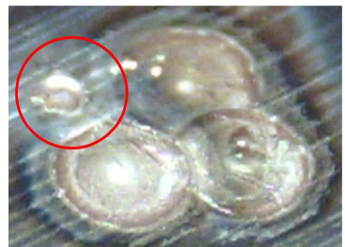
Figure 21.2. Electrode contamination can lead to small “explosions” that create craters in the workpiece.
