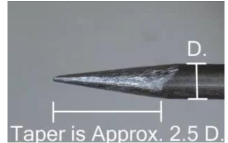
Figure 17.3. The electrode should be ground so that the taper is approximately 2.5 times the diameter.
