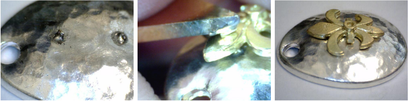
Figure 13.1. A weldment, or bump between parts to be welded, forces the electrical current to pass through a concentrated point (especially important for thicker parts). The smaller the bump tip diameter the more heat that can be generated at that point. This technique is also very helpful for welding dissimilar, conductive metals.
