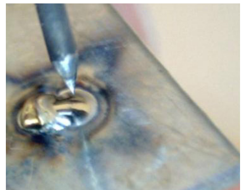
Figure 25.2. Placing the weld electrode on the edge of a bump will smooth away the bump as surface tension spreads the metal over the molten base material.
