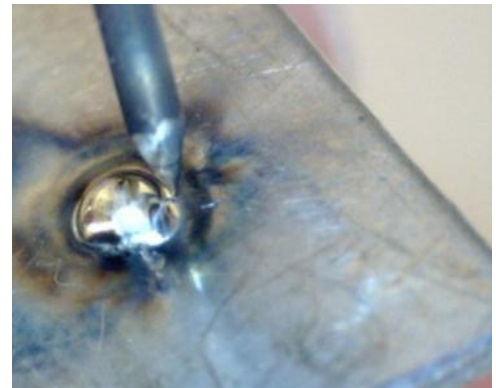
Figure 25.1. By placing the electrode between a high and low spot, the melting process will try and "flatten" the two, taking material from the high area and moving it toward the low area.
