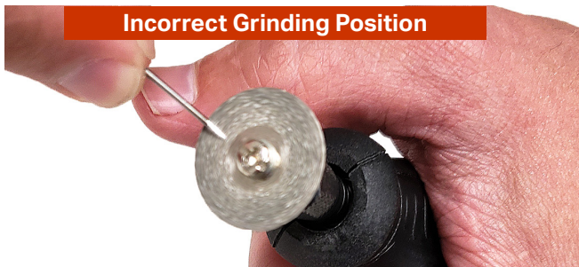
Figure 17.4. Always grind the welding electrode so that grind marks run parallel to the electrode shaft, as shown in the picture on the right.
