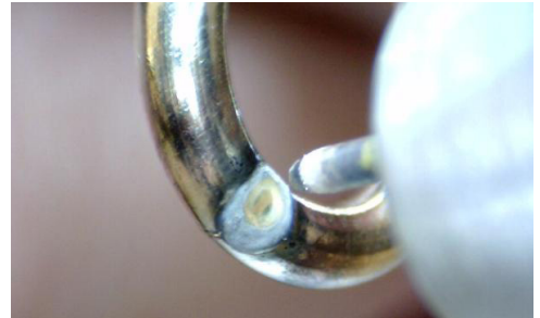
Figure 19.1. A blunt electrode tip can be helpful when making more powerful welds in silver to help overcome silver’s high liquid mobility by “un-focusing” the plasma over the entire flattened area.
