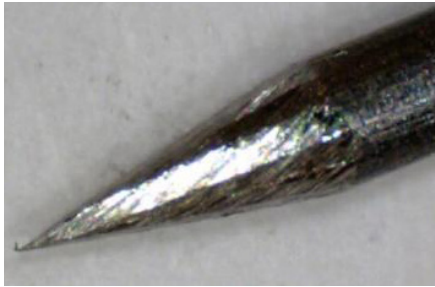
Figure 17.1. When grinding, make sure that grind marks run parallel to the electrode shaft.
