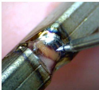
Figure 15.2. Using a 1.0mm electrode can weld at a variety of energies without overheating.
