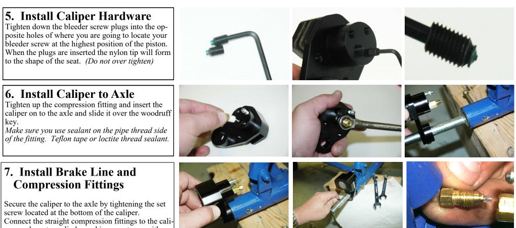
Connect the straight compression fittings to the callpers and master cylinder making sure to use either Teflon tape or loctite thread sealant on the pipe threads only. You do not need to seal the threads on the bleeder screw, bleeder screw plugs, or the compression fitting threads, just the pipe threads going into the caliper and the master cylinder. Using the "T" connecter, route the brake li
