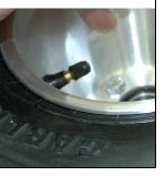
In 2021 we were unable to get our standard one piece welded rims that we have supplied since we started, however, we were able to source a new wheel that is very close but has a .500" deeper inside halve then our standard rim. This did not leave quite enough clearance for our caliper so with this rim we have to use the supplied hub spacer (59120) to push the hub away from the wheel .125". This will give enough clearance for the caliper to assure it will not make contact with the rim.
