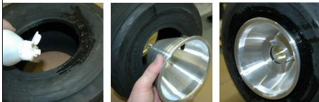
Tighten the bolts to the hub attach the flange nuts to the excess thread protruding form the back of the hub to secure the hub bolts for safety.
