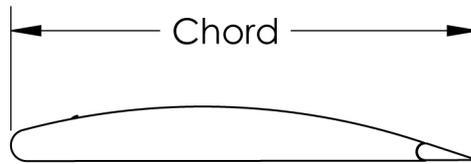
The chord position should be measured from the front edge of the wing to the aft side of the ailerons or flaps.
