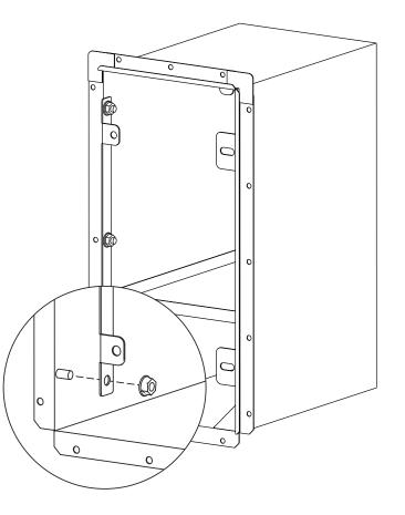
Mount the mounting clips on the right side of the rear box/sleeve. Please follow pictures 1, 2, and 3 for a detailed explanation on how to securely fasten the mounting clips (refer to the illustration on the right).
