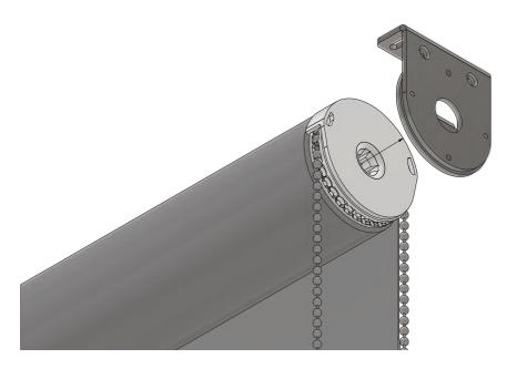
For a crank-operated blind, ensure the gear is engaged on the bracket in your desired orientation, then engage the pin in the end of the blind with the gear.
