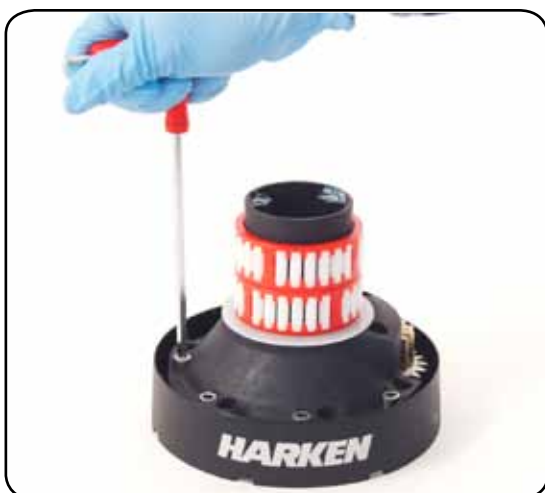
8. Unscrew the 6 hex screws n°16 (8Nm/70 in-lb)
