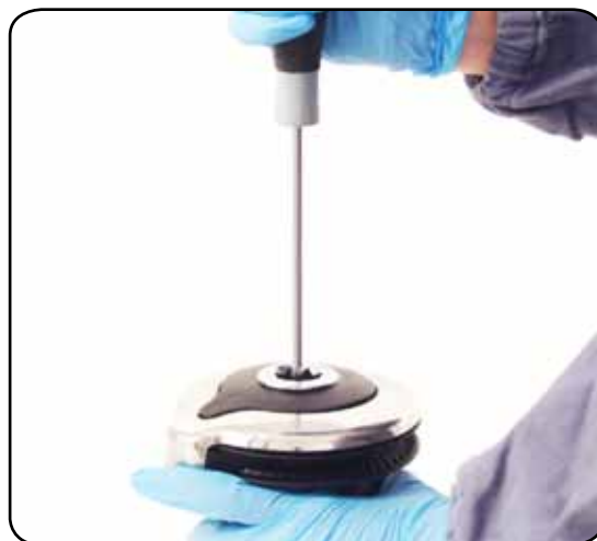
2. Unscrew the central screw ( \approx 2\text{Nm}/18\text{ in-lb} )
