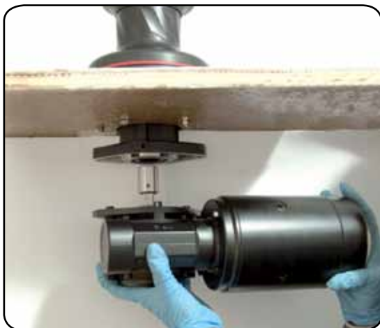
3. Position the reduction gear and motor
