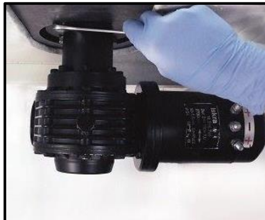
L. Tighten the four M10 screws (20Nm/177 in-lb)
