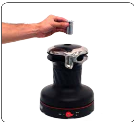
3. Slide off the assy socket n°35 and the cover n°19. Pay attention to the o-ring in the socket.
