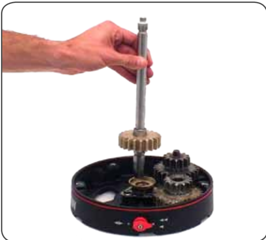
10. Slide out the central shaft n°24 and pay attention to the two balls n°26
