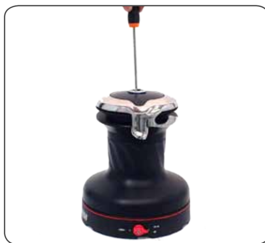
2. Unscrew the central screw ( \approx 2\text{Nm}/18\text{ in-lb} )
