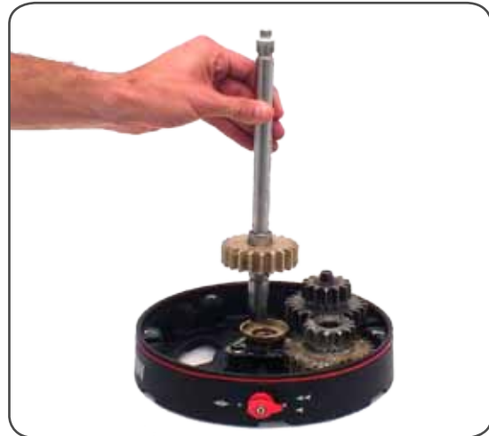
10. Slide out the central shaft n°25
