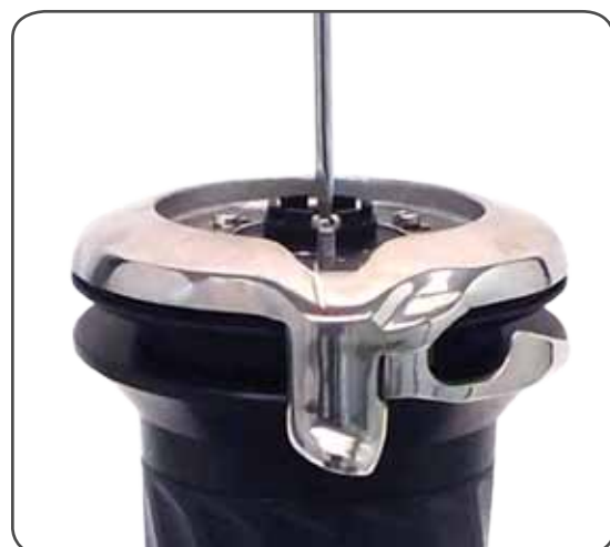
4. Unscrew the three screws n°42 ( \curvearrowright 4Nm/35 in-lb)
