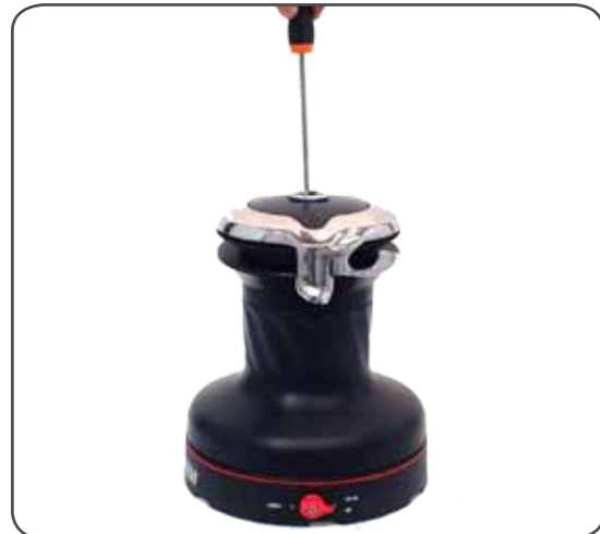
2. Unscrew the central screw ( \curvearrowright 2Nm/18 in-lb)
