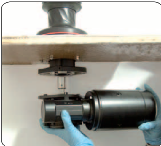
3. Position the reduction gear and motor
