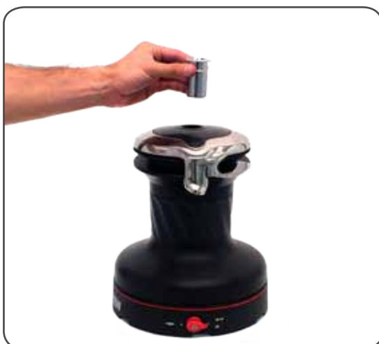
3. Slide off the assy socket n°38 and the cover n°19. Pay attention to the o-ring in the socket.
