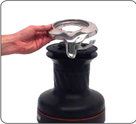
5. Remove the stripper arm n°48 by rotating and lifting it.
