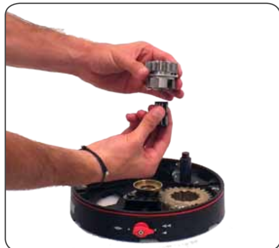
12. Remove the pawls carrier gear n°8 and slide out the 2 roller bearings n°9
