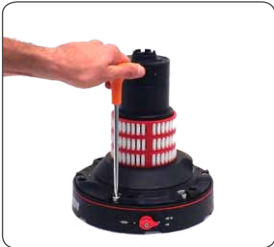
7. Unscrew the 6 hex screws n°14 ( \approx 20Nm/177 in-lb)
