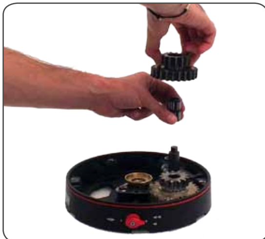
11. Remove the idler and pinion n°11 and slide out the two roller bearing n°12
