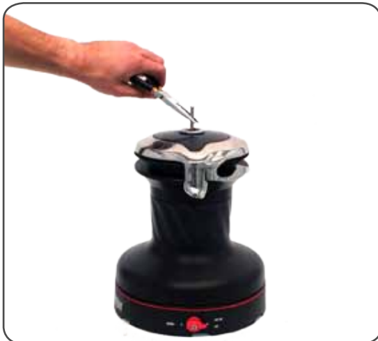
1. Pull out the disconnect rod n°22
