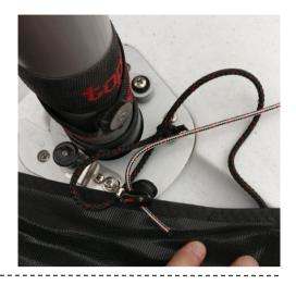
2.5 Pass the halyard through this pulley, found underneath the spinnaker bag at the bow. Then pass the halyard back underneath the bag towards the stern.
