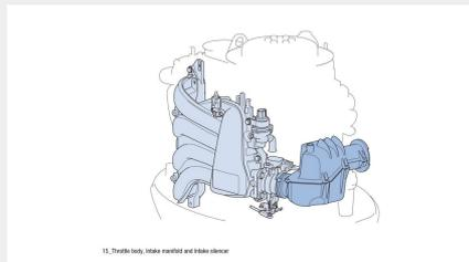
12. Throttle body, intake manifold and bubble cleaner
