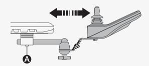
This is how you adjust the resistance of the rotational panel holder. Loosen or tighten knob  $\odot$  on the friction joint to adjust how easily the rotational panel holder can be pushed to either side.
