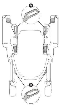
The wheelchair is equipped with four tie-down points used for transportation  $\blacksquare \checkmark \boxdot$ . Two in the front (**(()**) and two in the rear (**(()**).
