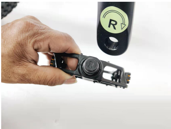
The pedal with letter R should be fixed on the right
