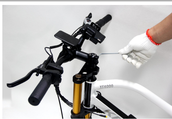
Tighten the bolts on the other side
