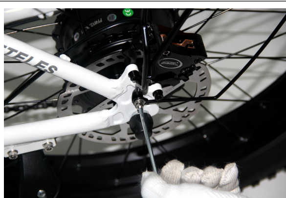
Tighten the two lower bolts on both sides
