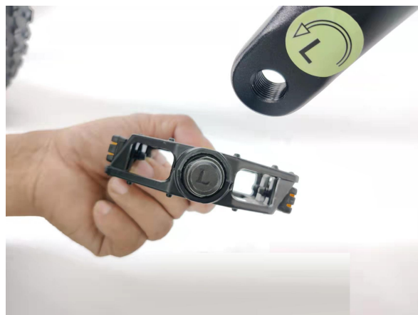
The pedal with letter L should be fixed on the left
