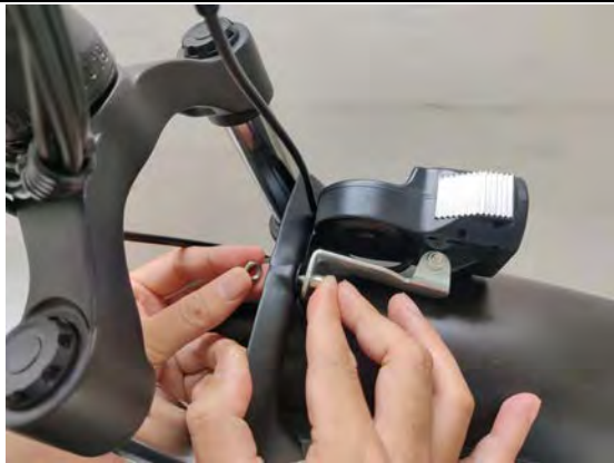
Use the bolt to join the headlight, fork arch and fender
