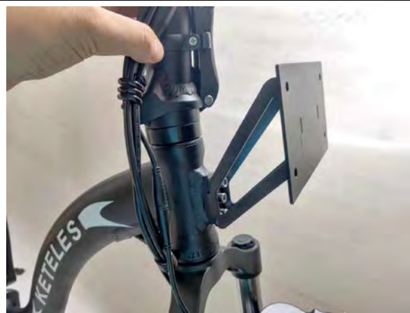
The headlight and front fender are fixed to the fork
