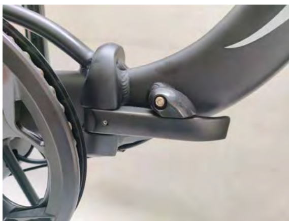
The safety switch and the frame folding quick release lever
