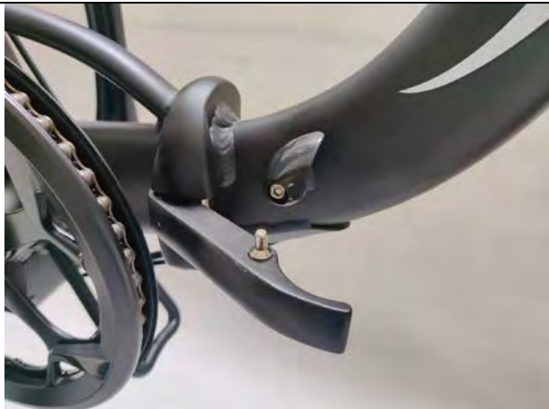
Pull the frame folding quick release lever outward
