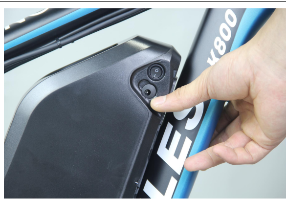
The charging port and the battery ON-OFF switch
