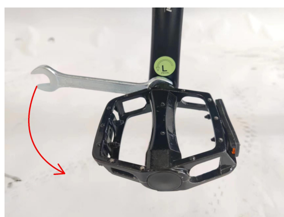
Turn spanner counter-clockwise to fix the pedal L
