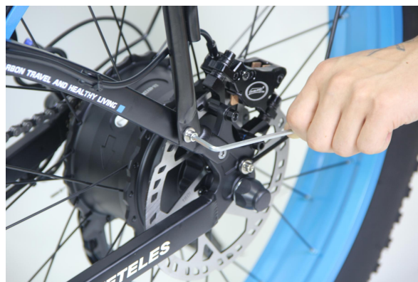
Tighten the two lower bolts on both sides
