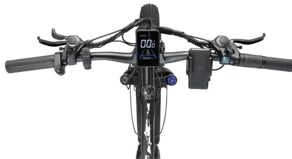
Multifunctional color LCD display in the middle . Press + or - can change speed grade .
