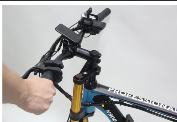
Fit the stem and handlebar together
