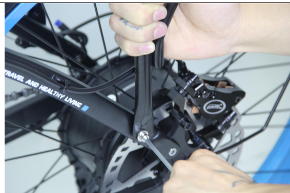
Tighten the two upper bolts on both sides
