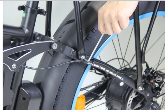
Tighten the two upper bolts on both sides
