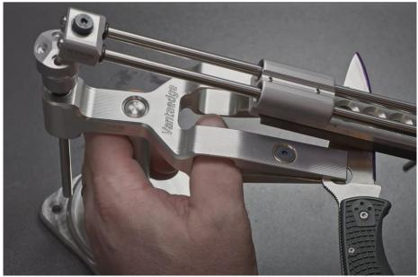
The other hand you push down the stainless holder and let jump up the angle head. Stil push down the stone holder and make movement up and down the stone along all the edge, when one side is finished, take away the stone holder including angle head and turn the clamp around and sharpen the other side too. Start with coarse stones and go to fine stones.
