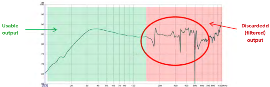
Figure 5. On-axis response of cone diaphragm speaker. Only part of the frequency range is usable, the region where breakup occurs (red) must be filtered away.
