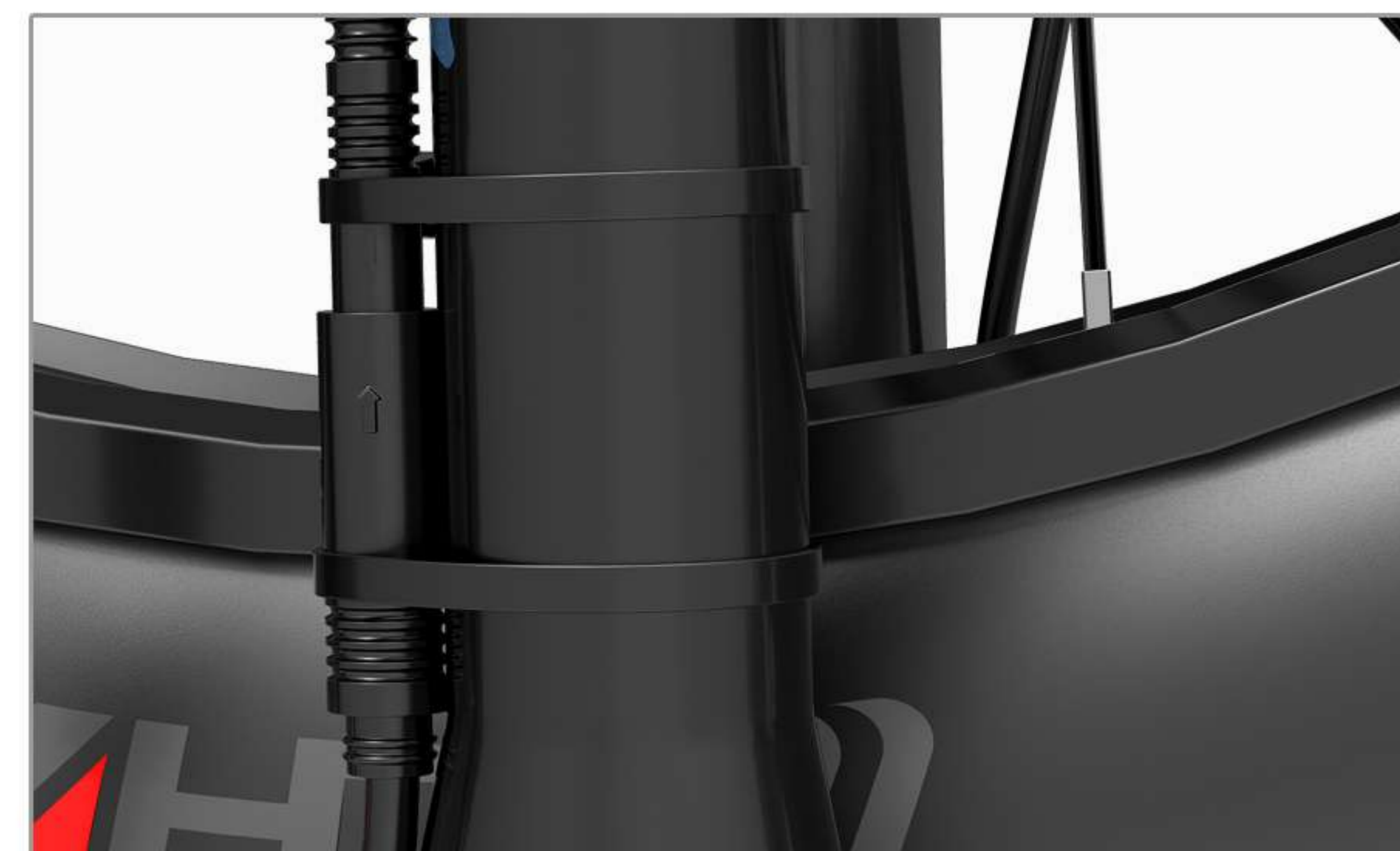
09 After the front wheel motor wire is connected, use a tie to fix the wire on the front fork.
