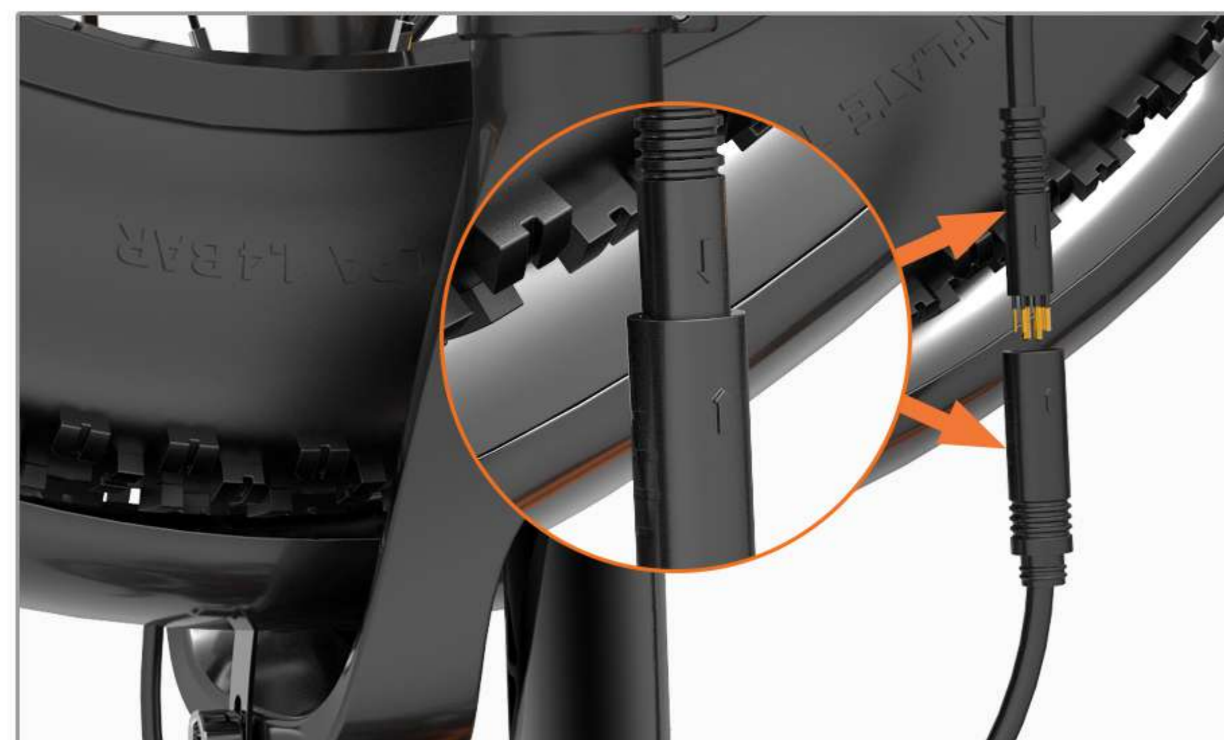
08 Connect the front wheel motor cable plug *Pay attention to the alignment of arrows between lines when linking
