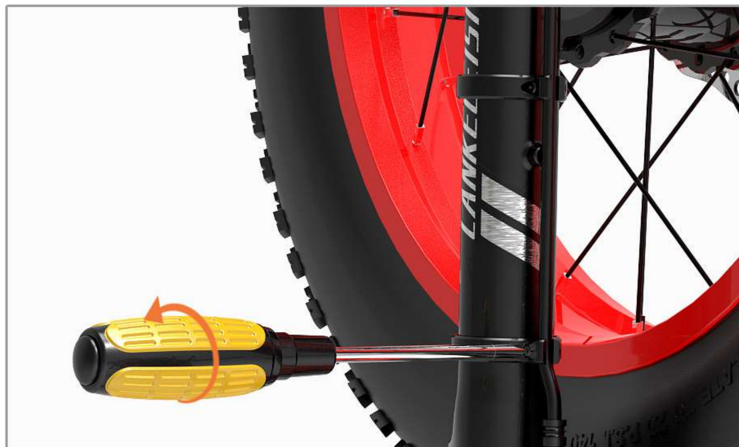
10 Fix the line on the line buckle and tighten the screw
