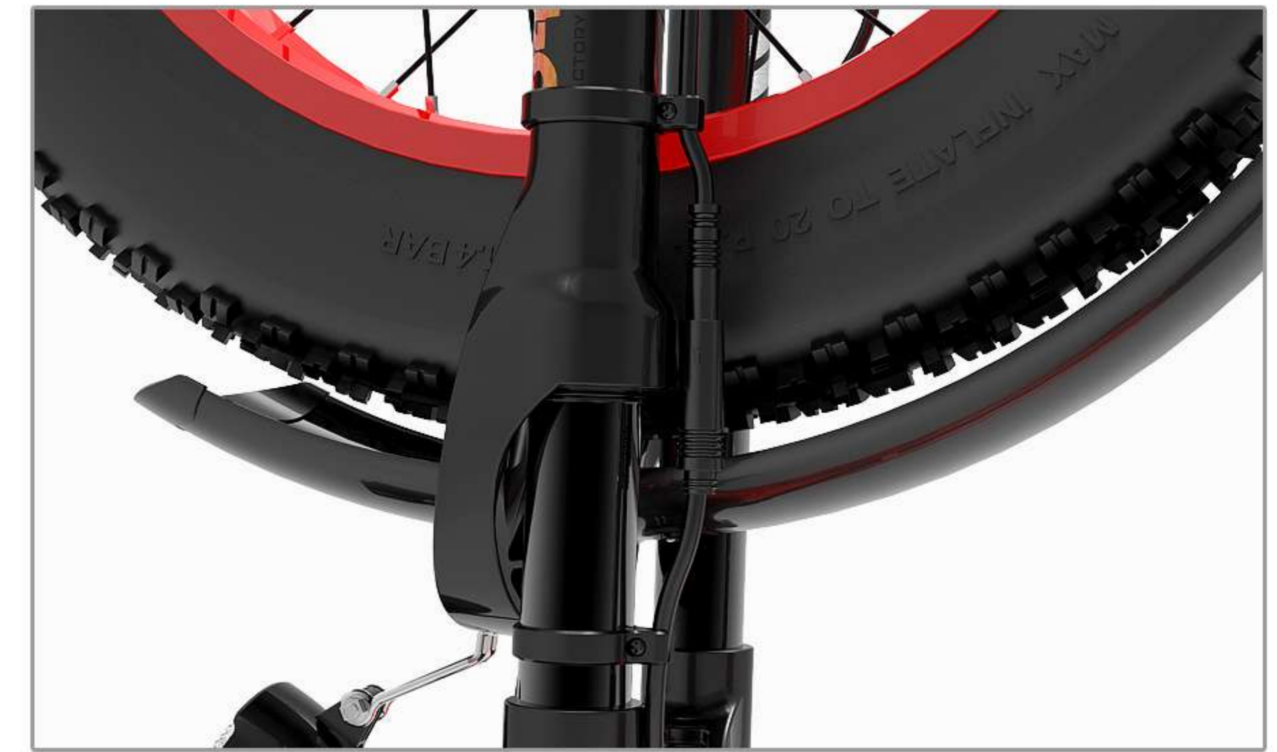
09 After the front wheel motor wire is connected, use a tie to fix the wire on the front fork.
