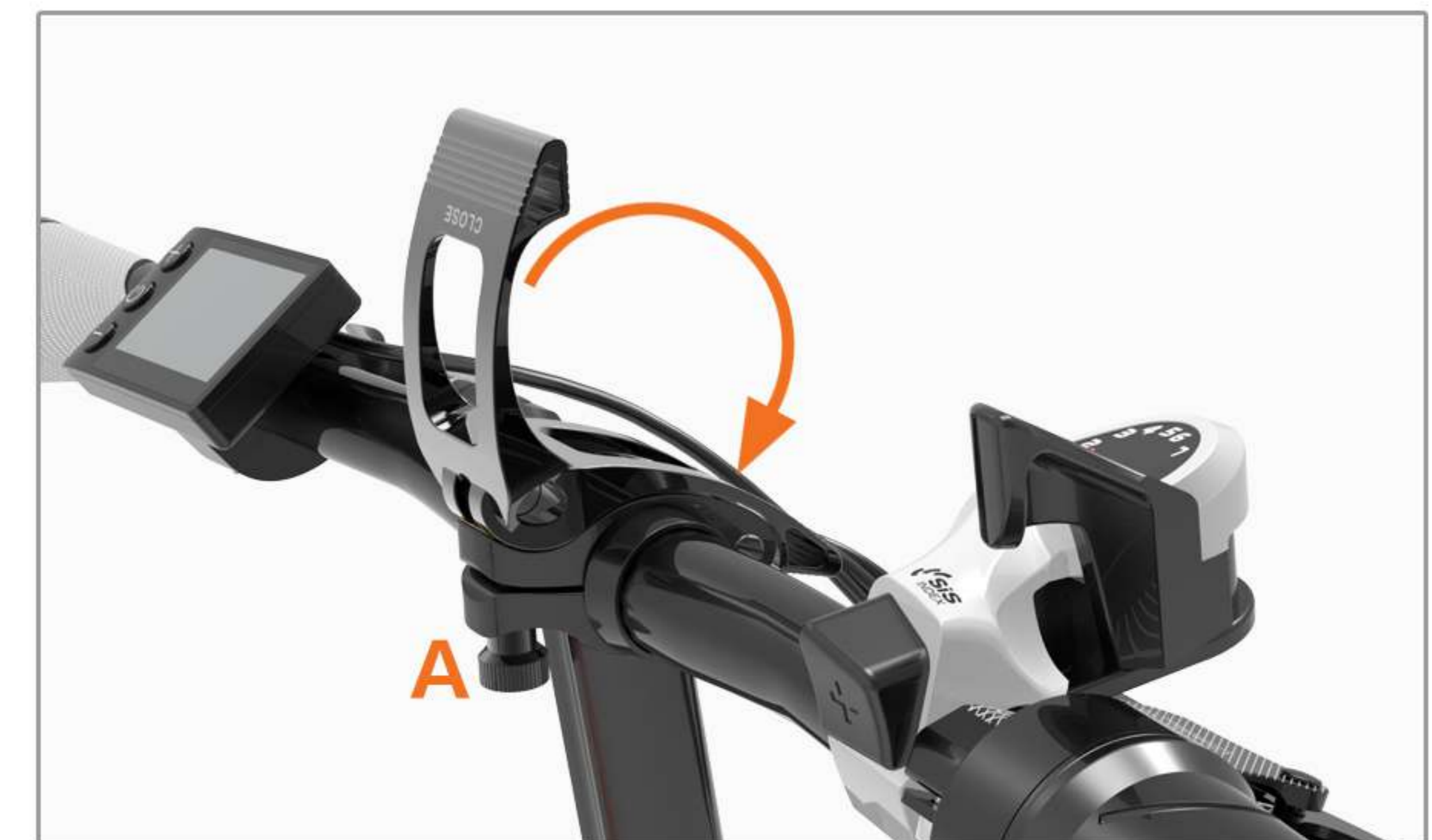
06 Tighten the quick release rod A:tighten
