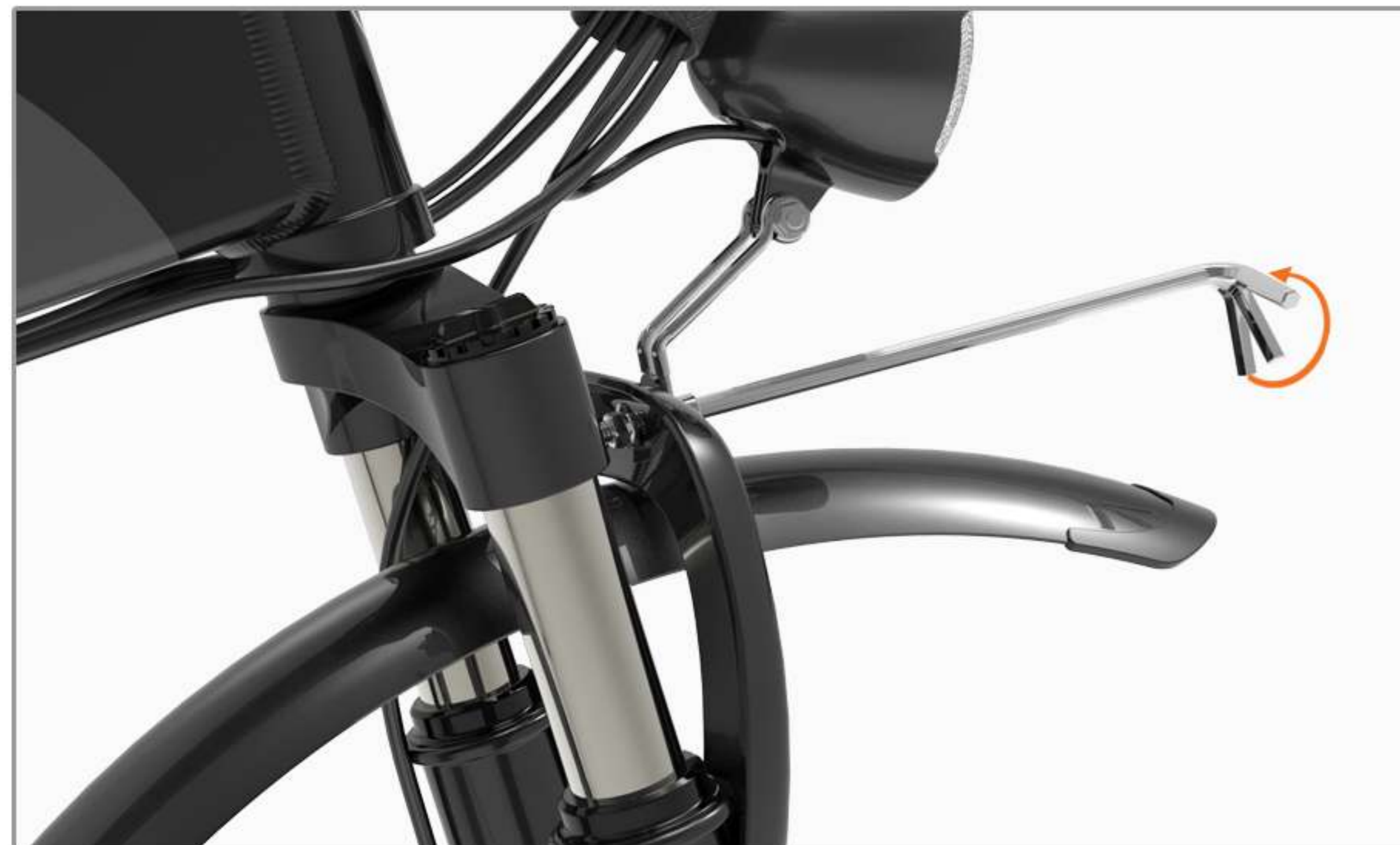
01 Fix the mudguard with the same screw as the front light
