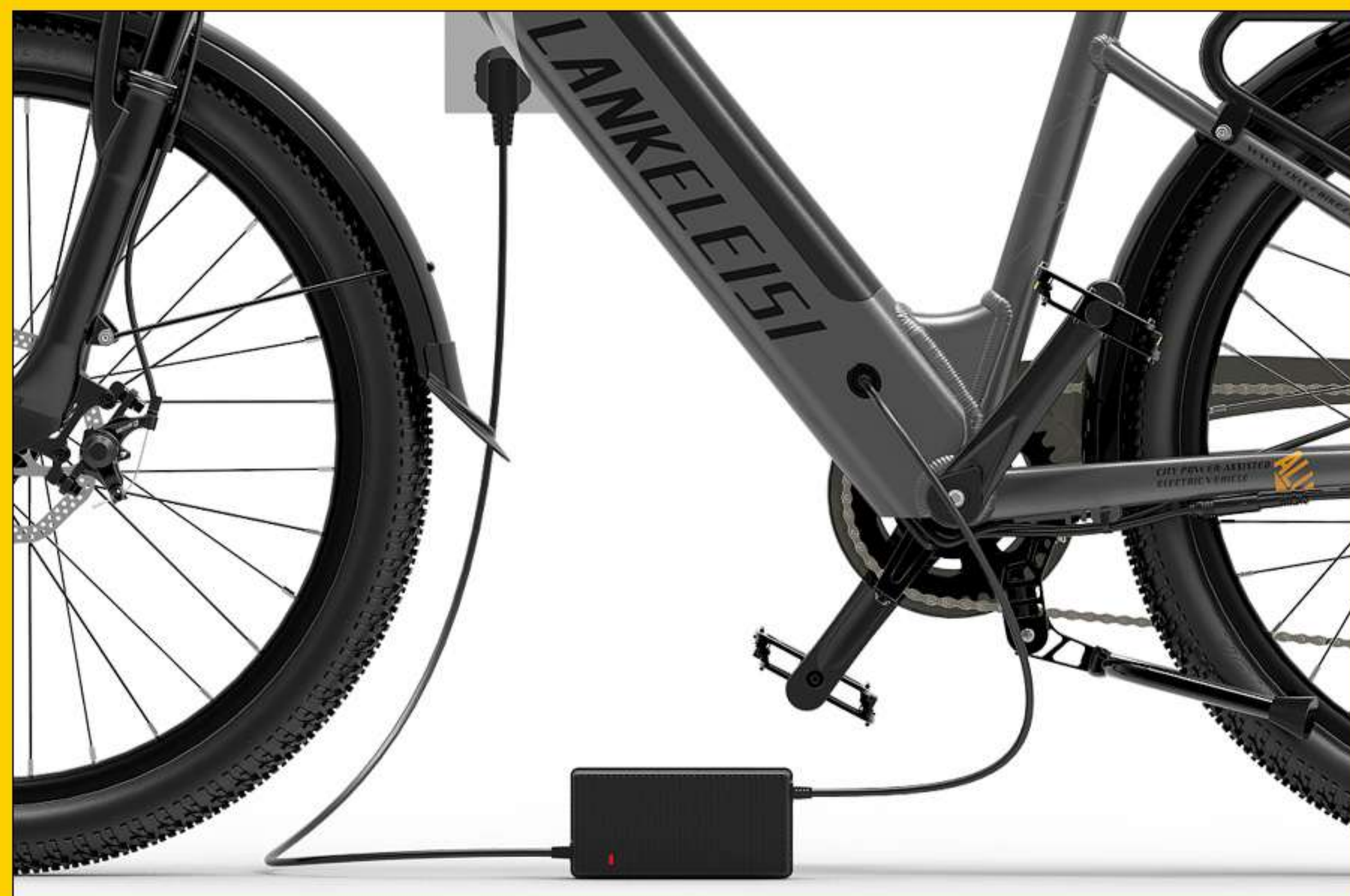
A. Recharge the battery on E-Bike directly
