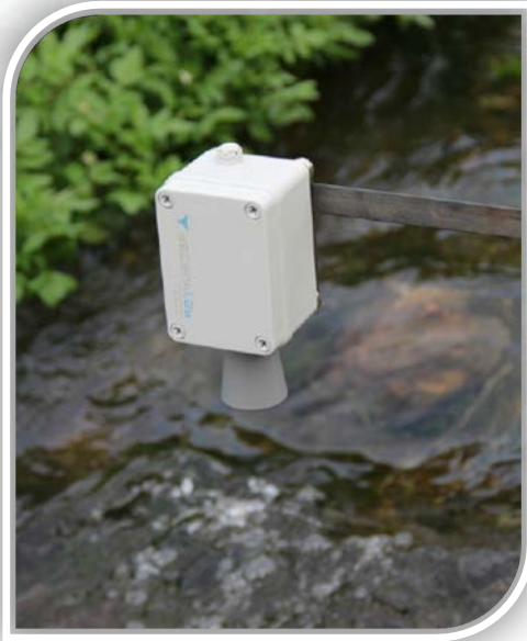
Ultrasonic water level sensor – North Tyne
