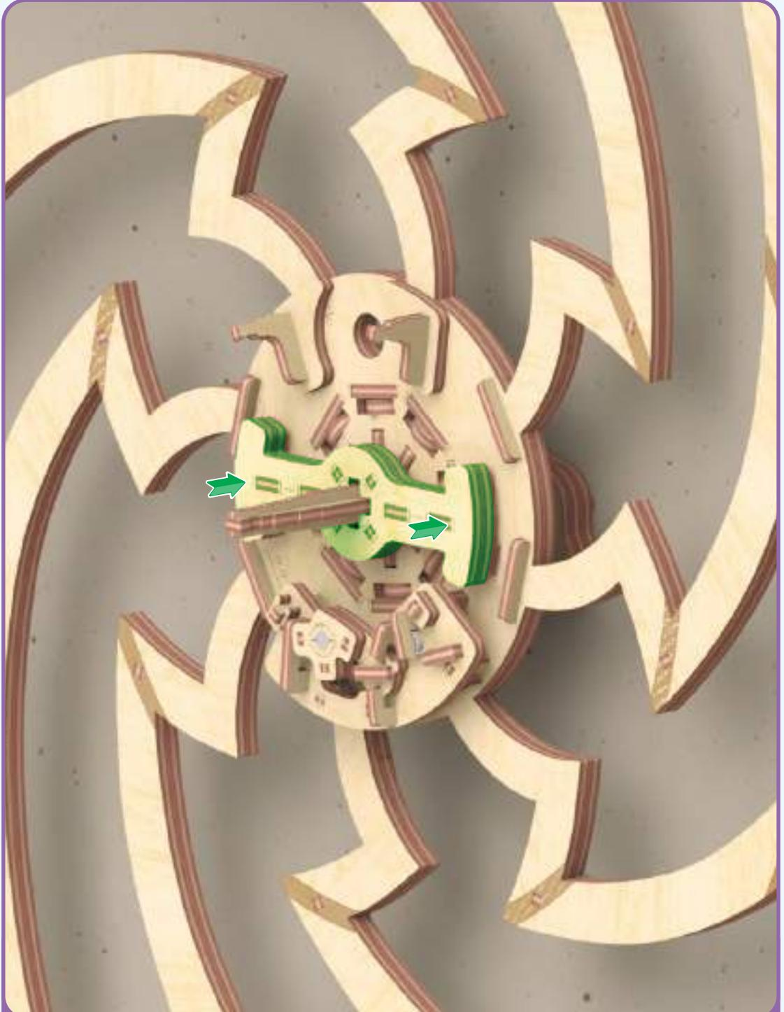
**EN** Apply even force to the base of the spinner and the bearing at the same time when mounting the spinner on the axle. The spinner must be installed vertically, without tilting forward or backward.
