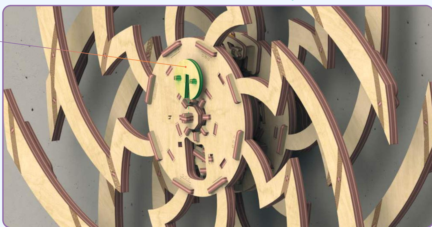
**EN** Mechanism explanation: when the front and rear ratchets converge, the front one should engage with the ratchet wheel and the rear one should disengage from the ratchet wheel after the front ratchet turns the ratchet wheel slightly.
