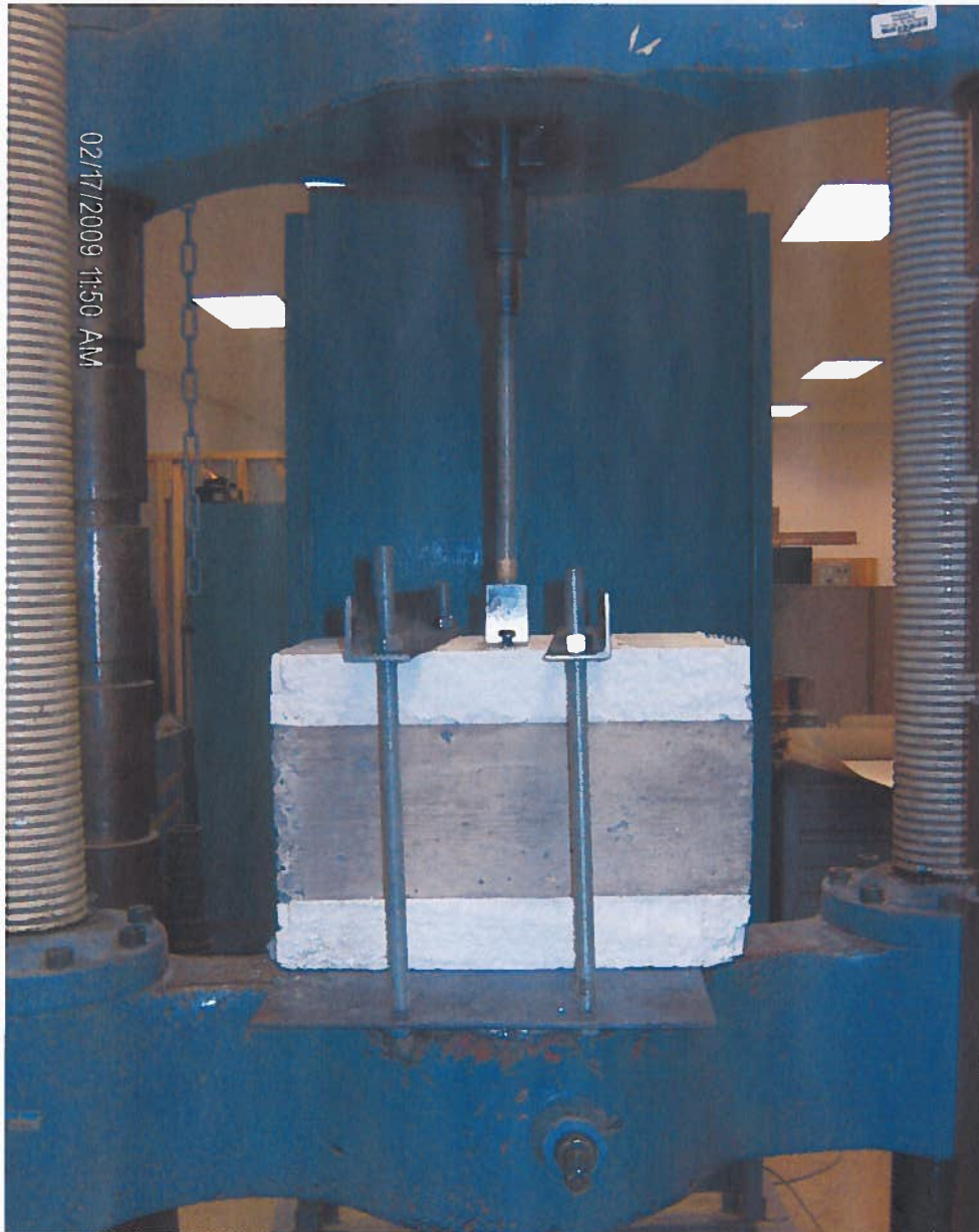
Photograph No. 11: Showing test set-up for screw and nail withdrawal test using Baldwin Universal Testing Machine.
