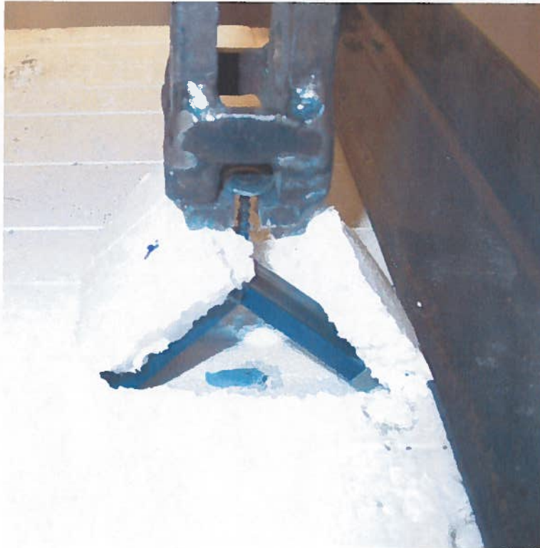
Photograph No. 16: Showing the web fracturing during a screw withdrawal test.
