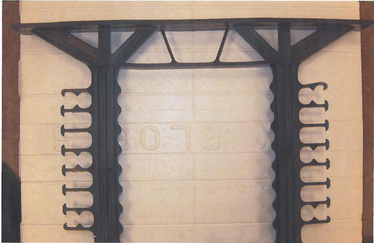
Photograph No. 1: Showing a typical web specimen.
