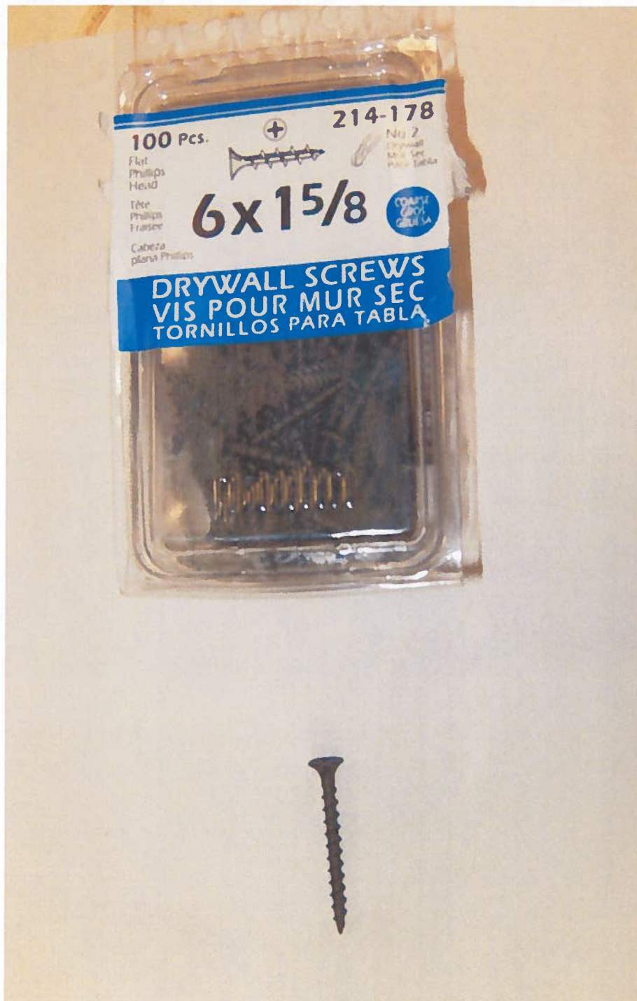
Photograph No. 5: Showing Paulin Fasteners 6 x 1-5/8 Coarse Drywall Screw Number 214-178.
