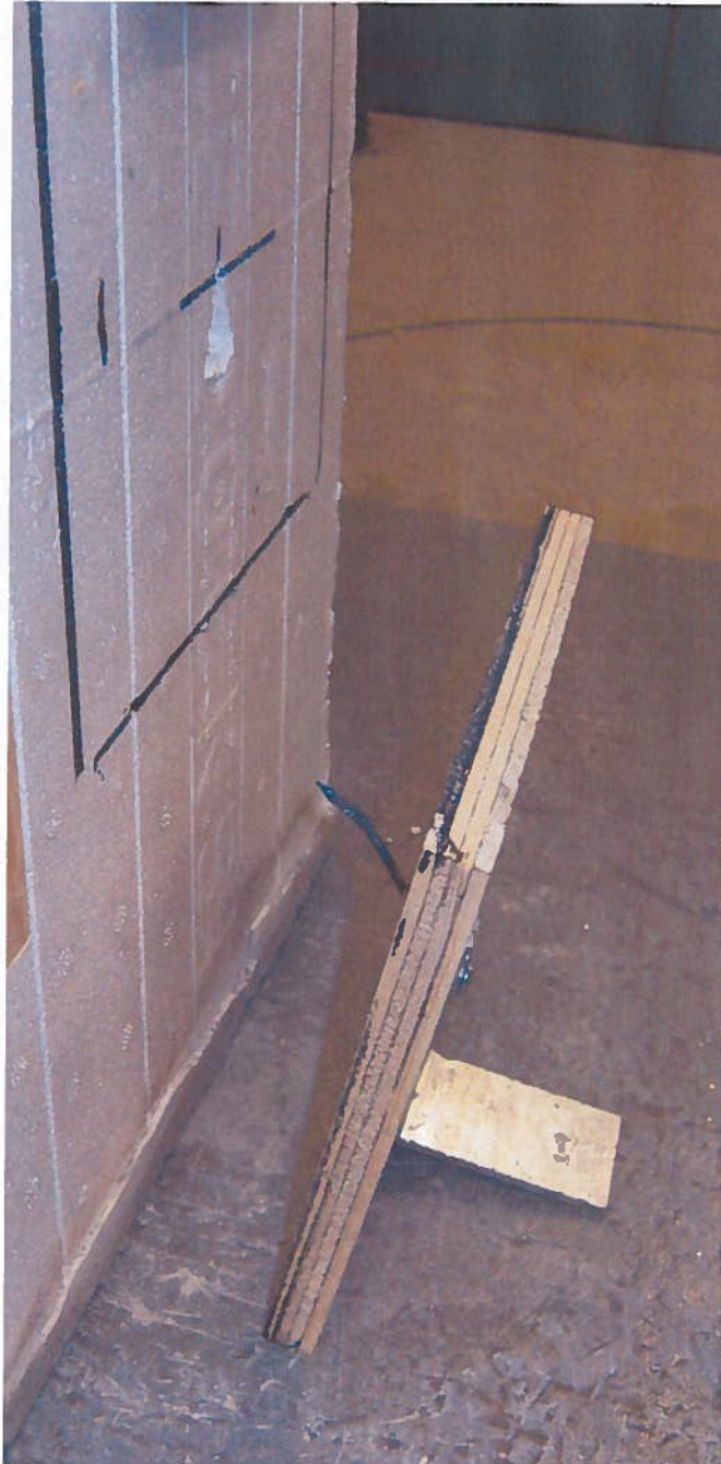
Photograph No. 15: Showing a typical 2" dry wall nail bending and pulling out of the web due lateral fastener resistance tests.
