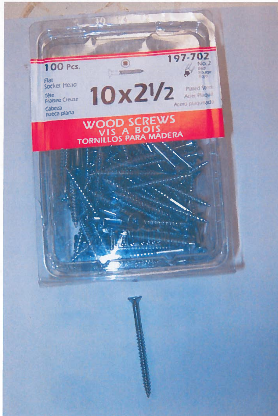
Photograph No. 7: Showing Paulin Fasteners 10 x 2-1/2 Wood Screws Number 197-702.
