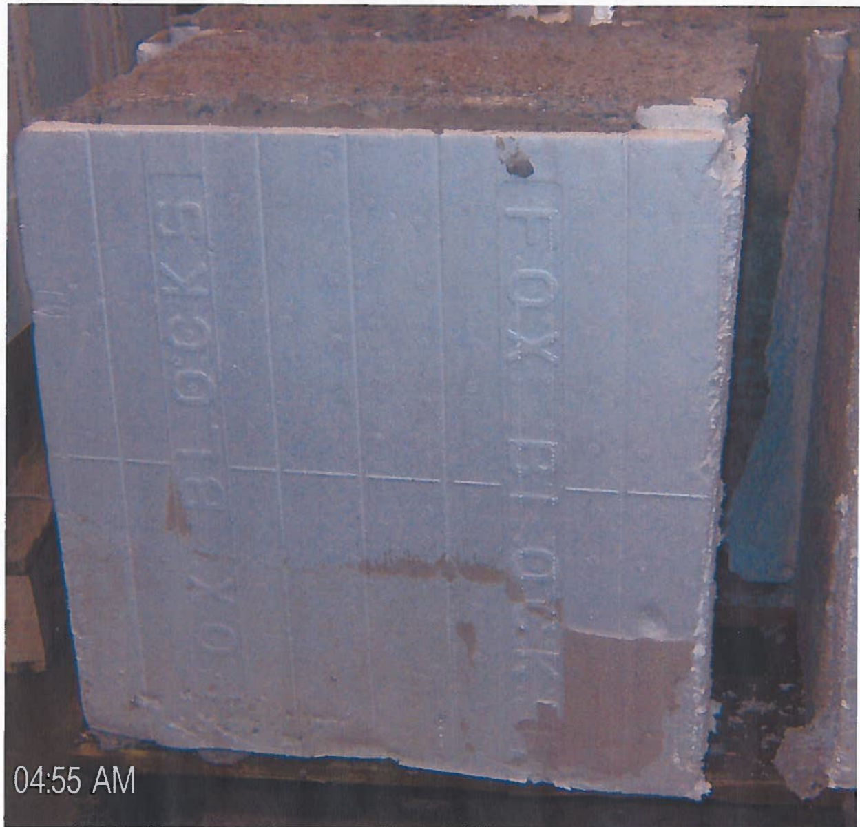
Photograph No. 3: Showing a typical insulated concrete form test specimen.
