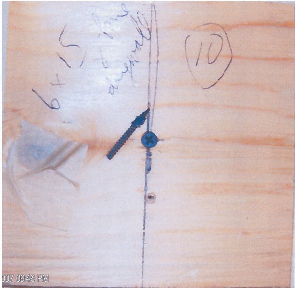
Photograph No. 14: Showing a shaft of a drywall screw fracturing at the foam to plywood interface due lateral fastener resistance tests.
