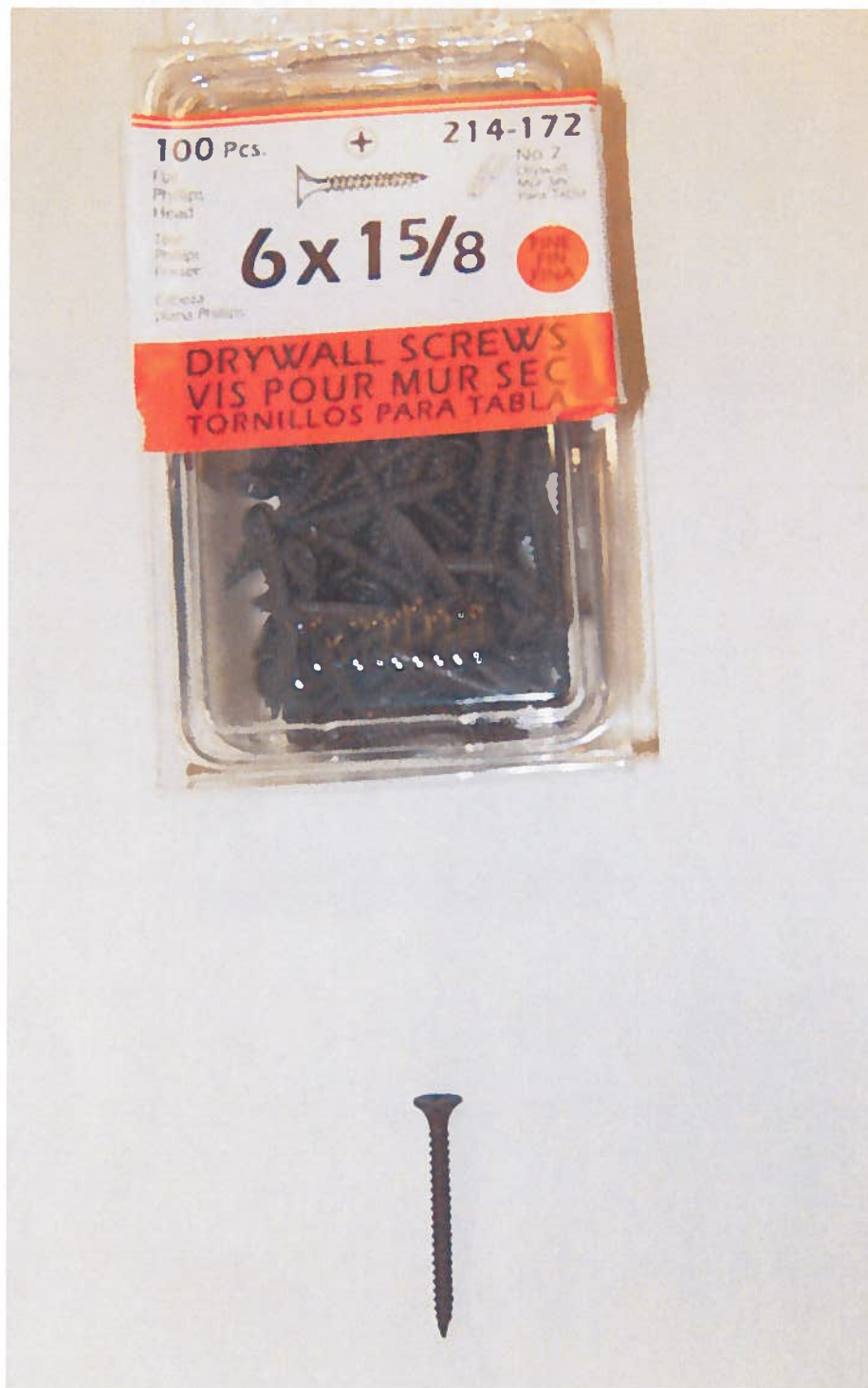
Photograph No. 4: Showing Paulin Fasteners 6 x 1-5/8 Fine Drywall Screw Number 214-172.
