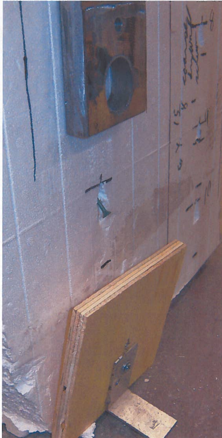
Photograph No. 13 Showing a deck screw having pulled through the plywood during a lateral fastener resistance test.
