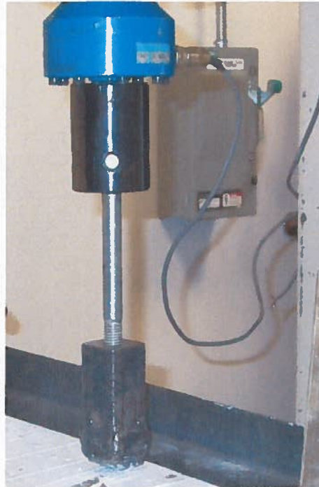
Photograph No. 10: Showing test set-up for screw and nail withdrawal test using Satec Unidrive Testing Machine.
