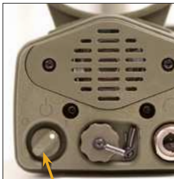
On/Off Switch (shown in On position)
