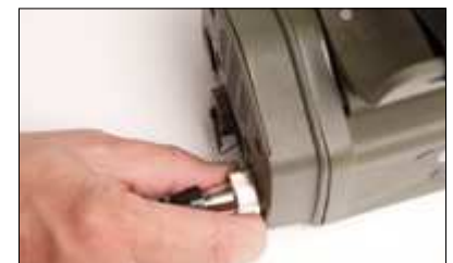
Hand-tighten connector collar.
