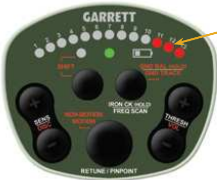
Three red LEDs to the far right indicates maximum target signal strength.
