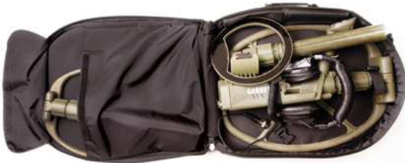
Figure 6: ATX with Deepseeker coil attached + DD coil + 8" mono coil + headphones. Note: close velcro flap to secure DD coil.
