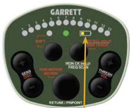
Low Battery Indicator
