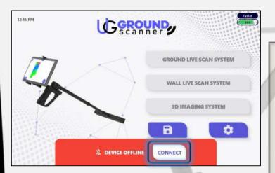
Connection icon: to establish a Bluetooth connection between the tablet and the imaging sensor.
