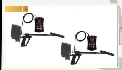
Plug the battery into the socket on the arm
