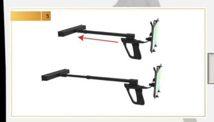
Extend the arm by releasing the lock in the middle
