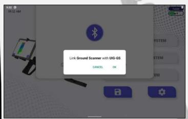
Tap the connection icon to set up pairing between the tablet and the imaging sensor.
