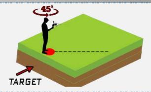
Measure the distance between the antennas reversing back and the target center point.
