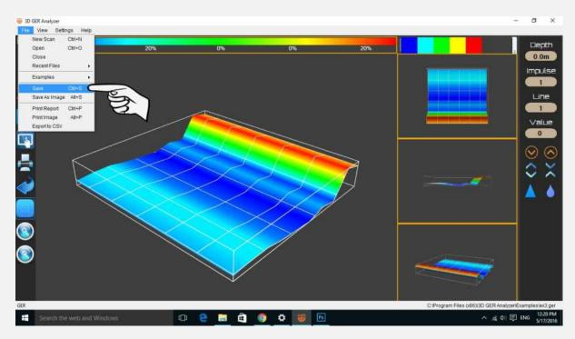
After you finish the scanning you can save the scan on the tablet as a project to be able to analyze again also you can save it as a photo
