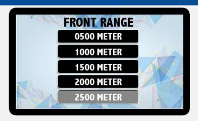
After selecting the Front Range, the search screen will appear which contain an indicator, which will guide you directly to the target. Make sure that the antenna is pointing ahead
