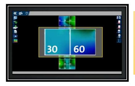
These criteria also apply to voids, i.e. if two squares are shown in blue with varying values by a large difference (i.e. 20 to 30 points), this indicates that one of these squares is a void and the other is a rock, this means that the higher value is a void and the lower value It is a rock.
