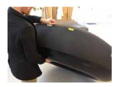
3. Lift the Tube with cover where you can see the flagtag. The valves are located near the flagtag.
