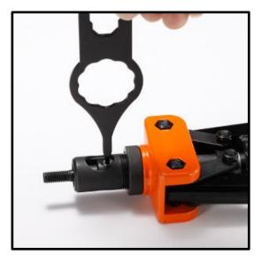
Use the sharp point of the spanner to detach the cross pin.
