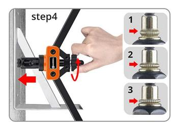
Repeat Step 2/3/4 at least 2-3 times to ensure that the nut is fully tightened.
