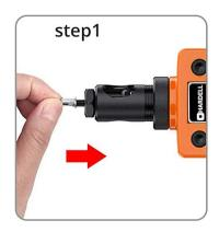
Install the nut on the mandrel, make sure the arms are completely opened.
