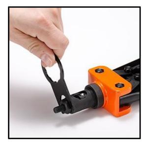
Remove nosepiece by unthreading the nosepiece counterclockwise. This can be either by hand or with the spanner if too tight...
