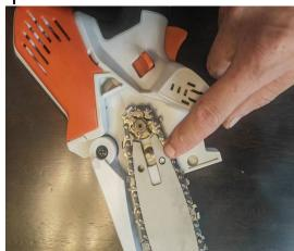
Align the corresponding hole position of the guide plate with the installed chain to the machine.
