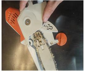
Remove the guide cover, guide plate and chain.
