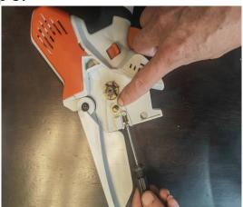
Use the provided screwdriver to turn the screw forward so that it can align with the guide plate hole.
