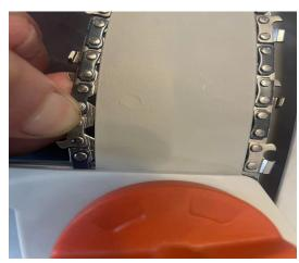
Install the guide cover back, and adjust the knob to tighten the chain with the provided screw/driver. The tightness of the chain should be left at 1-3mm as picture 2b.
