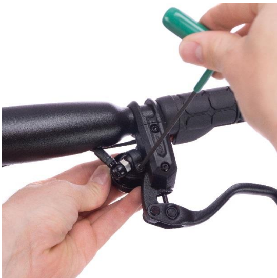
Tighten the bell mounting bracket with a Torx T10 to 2-3 Nm.
