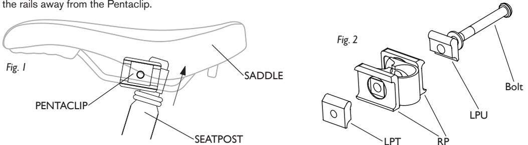
The Pentaclip can now be taken apart and the plates MCP and clamp band faces CBF degreased (fig. 3). Once the parts are clean and dry the Pentaclip can be reassembled with the clutch-plates fitted into the rail-plates (RP) in the order shown below. Plates MCP should be fitted with the formed 'ears' offset towards the outside of the bike (in order to engage fully with the rail-plates RP). The plates FCP may be a tight fit on the square splines.
