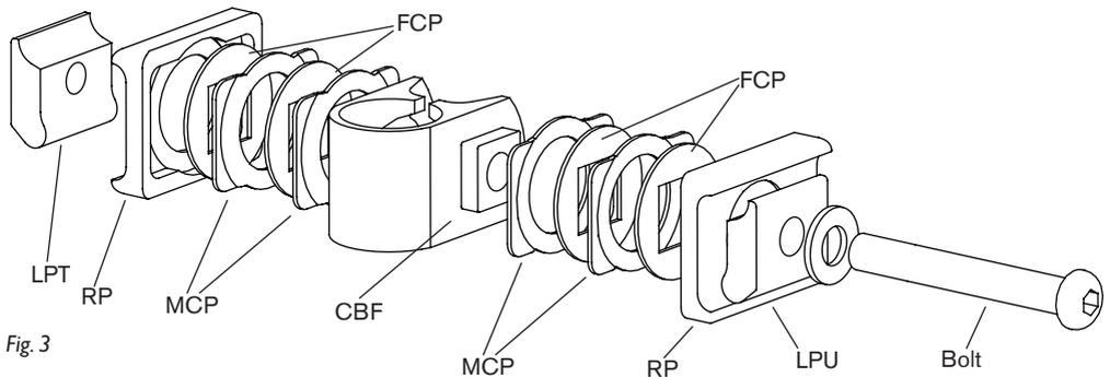
Refit the saddle to the Pentaclip and slide onto the seatpost, positioning it half way up the small diameter of the seatpost. Gently tighten the Pentaclip bolt with a 5mm hex key, leaving the assembly loose enough to adjust the saddle position. Ensure that you have the Pentaclip in the correct orientation and the saddle position and angle is correct. Once the saddle position is set, tighten the Pentaclip bolt to 15Nm.
