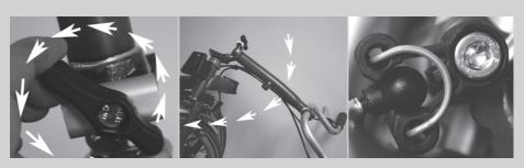
**Step 4**Undo the hinge clamp and swing the handlebars down alongside the front wheel and engage in the clip; alternatively, let the handlebar drop into position on its own.
