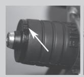
In the "locked" position, the rear frame will remain connected to the main frame when the bike is picked up.
