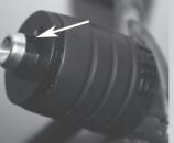
In the "unlocked" position, the rear frame will drop down when the bike is picked up.
