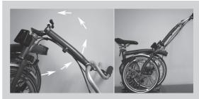
Step 2a Unfold the handlebar into the upright position as shown.
