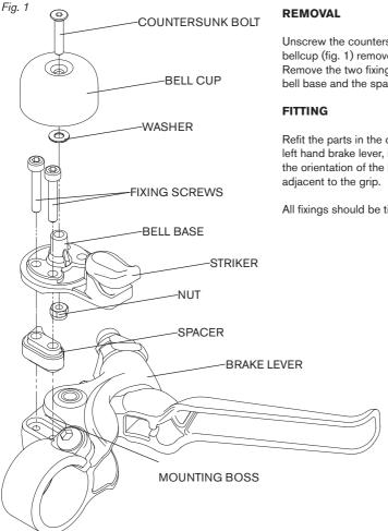
Unscrew the countersunk bolt in the centre of the bellcup (fig. 1) remove the bolt, bell cup and washer. Remove the two fixing screws and then remove the bell base and the spacer from the brake lever.
