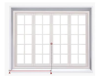
**T-Post position** is in the middle of width of window architrave.
