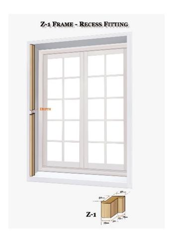
Z Frame - Minimum Depth required 38mm
