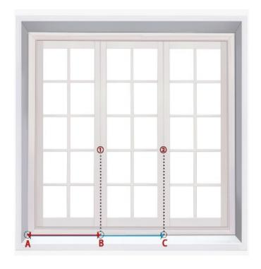
**T- Post 1 position:** from the left edge of the window reveal (A) to the middle of window frame (B) as shown on the picture.
