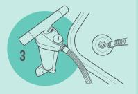
Attach the hose to the INF port on the pump.
