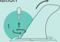
Remove the fin by loosening the screw then sliding the fin out of the channel. Be sure to also remove the square nut.
