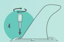
Tighten screw in front hole into square nut.
