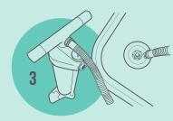
To fully deflate, attach hose to pump using **DEF** port. Use "double action" setting for fast deflation.
