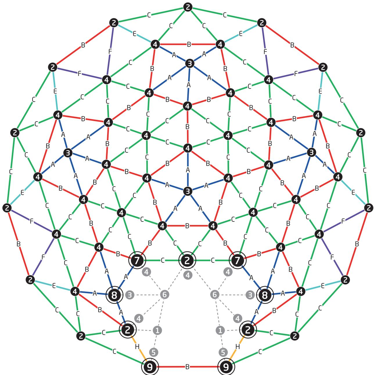
To convert your Garden Igloo to a summer canopy, first remove the parts listed on the left and replace the parts listed on the right (as it is shown in the above figure).
